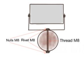
• Each pole will be carried into place by the Crew and be prepped by Install team (5 Crew). Poles will be drilled at the top and Speakers will be attached with Bolts - washers and safety Nuts. (Picture to the left)
