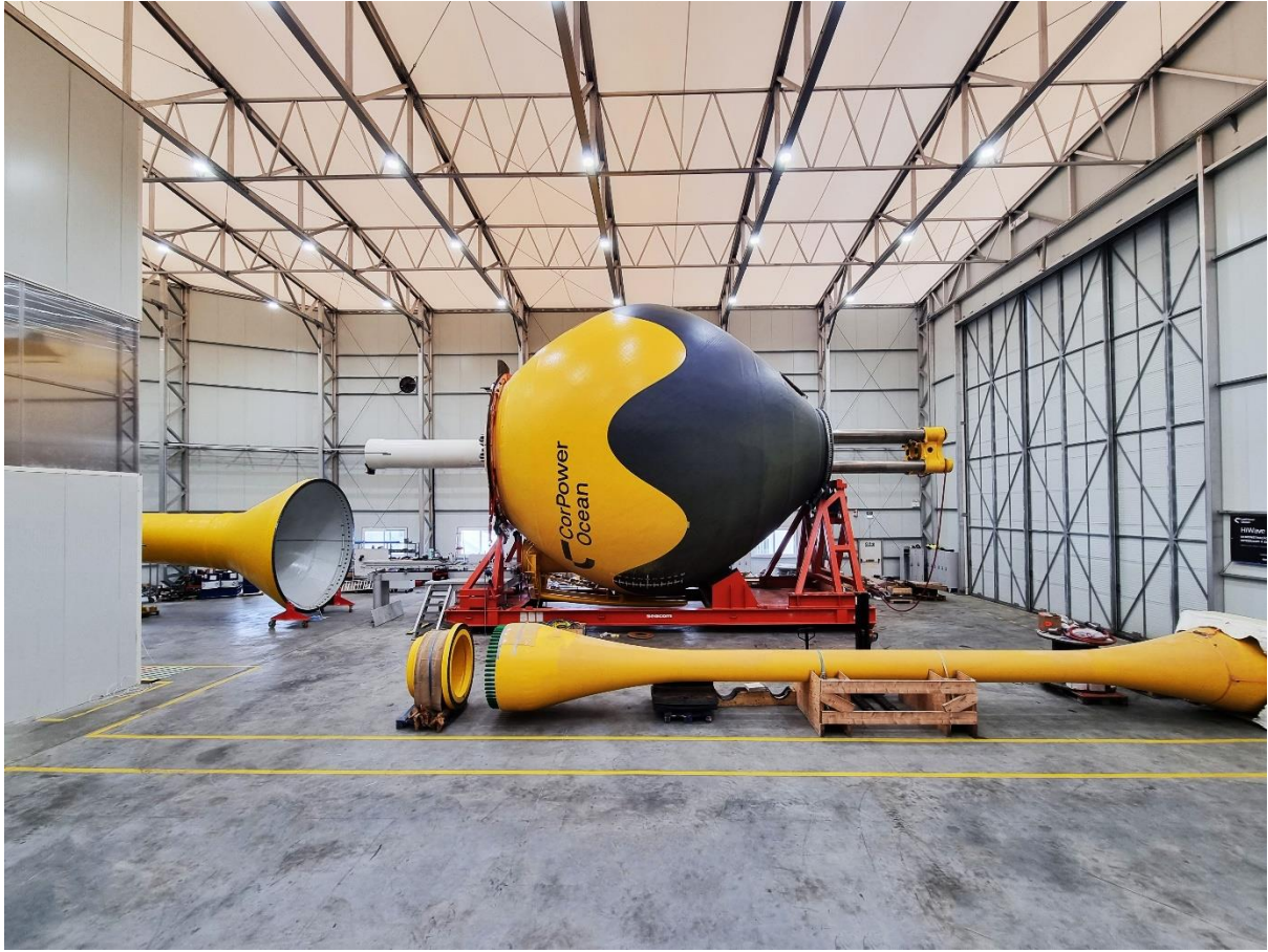
Figure 3. Corpower WEC with PTO mated in the composite hull, top shroud, and mooring rod in foreground
