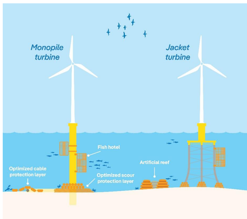
Figure 1.1 Illustrative image of potential nature positive options to show how they can be integrated into the design of the windfarm
