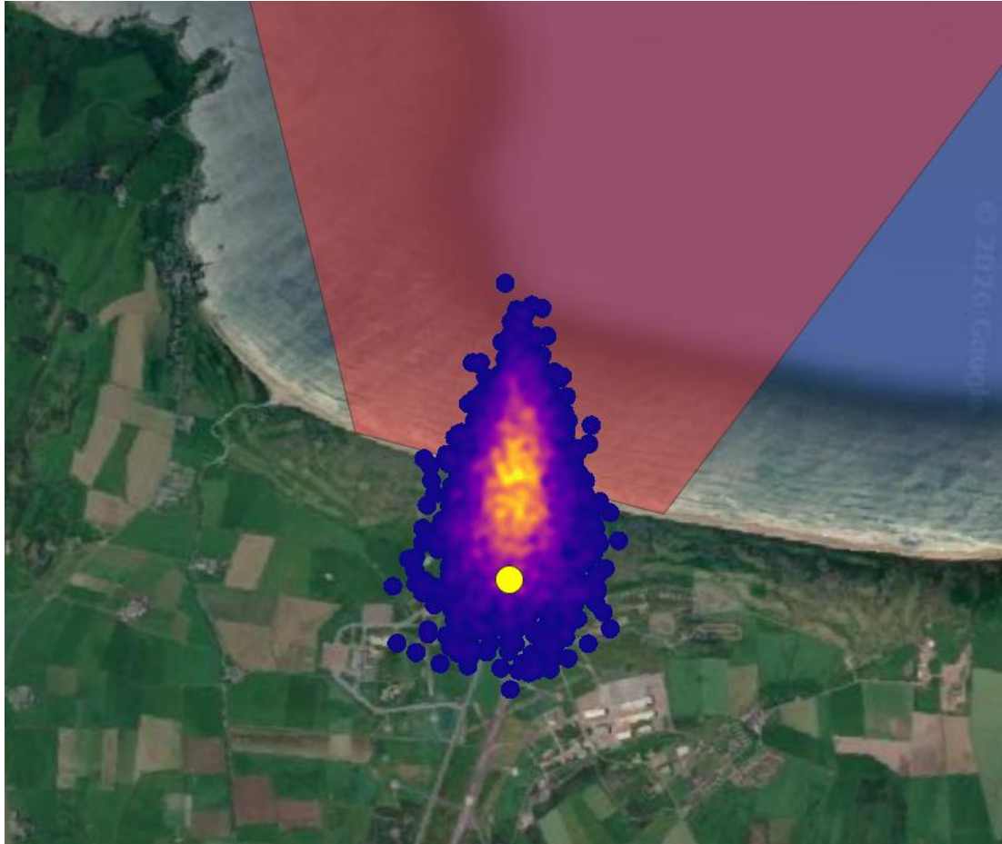
Figure 5 - Main-at-apogee Recovery Scenario
