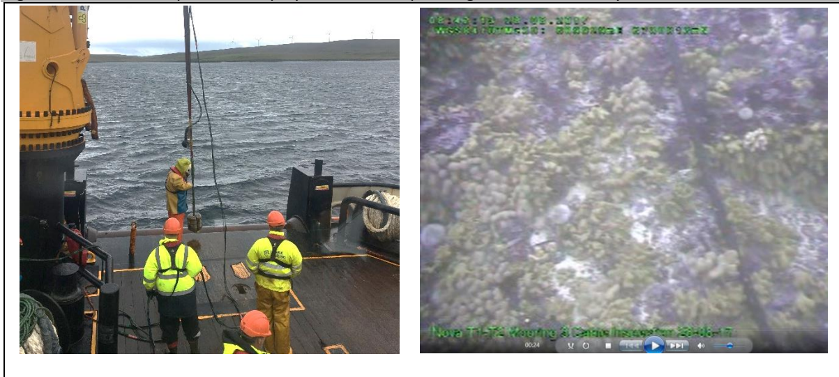
Figure 13: Multicat drop camera deployment and sample image from cable survey
