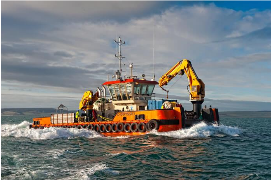
Figure 5.2 Representative turbine deployment and retrieval vessel
