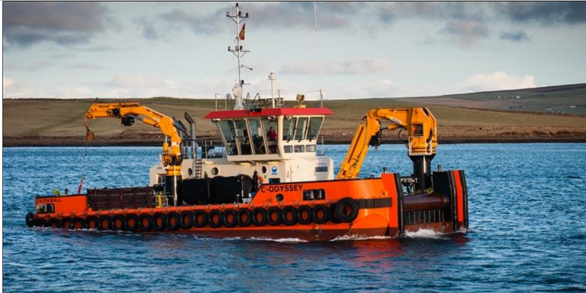
Figure 9: Representative turbine deployment and retrieval vessel (Leask Marine C-Odyssey)
