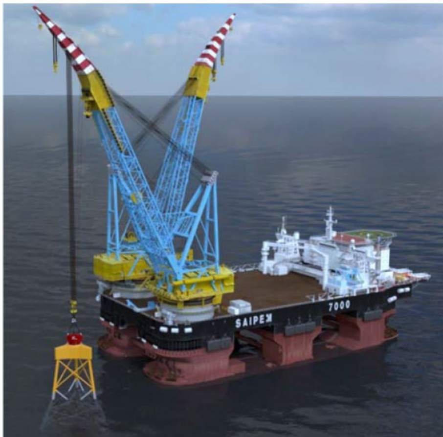
Figure 6-6: Deployment of the jacket from the SSCV
