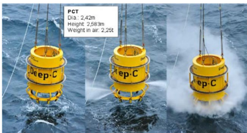
Figure 6-5: Pile cleaning tool
