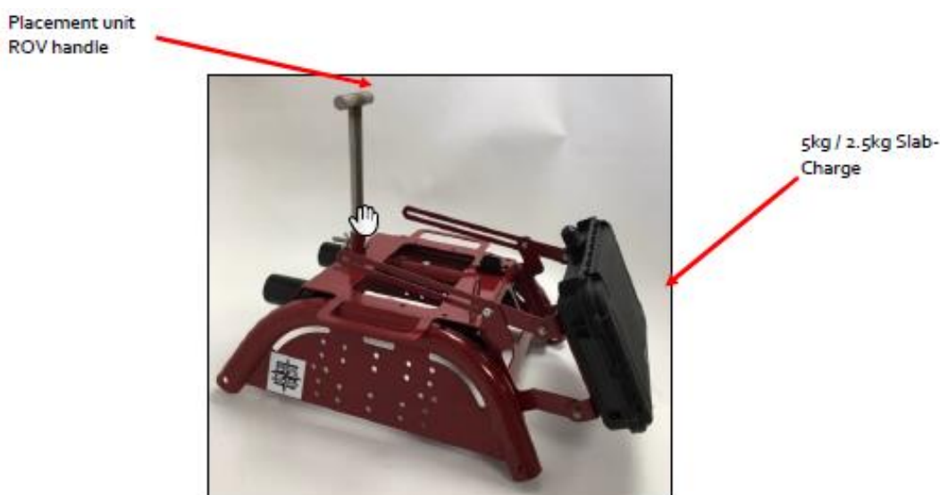
Figure 3 – Equipment used for UXO clearance activities
