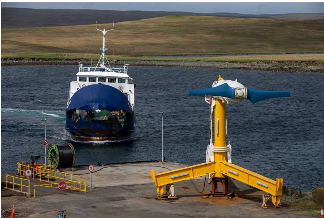
Figure 5-3 The Nova M100-D turbine prior to deployment in Bluemull Sound
