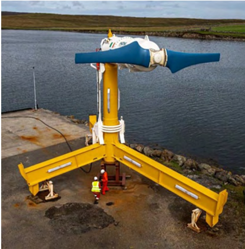
Figure 1-2 Nova’s M100-D direct drive tidal stream turbine on the quayside in Shetland
