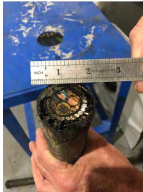
Figure 5-5 Typical subsea cable cross-section
