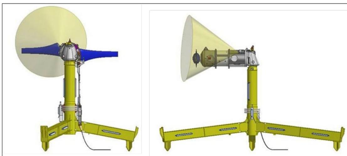
**Figure 4. Turbine-mounted subsea camera system for turbines in the OCEANSTAR Project.**
