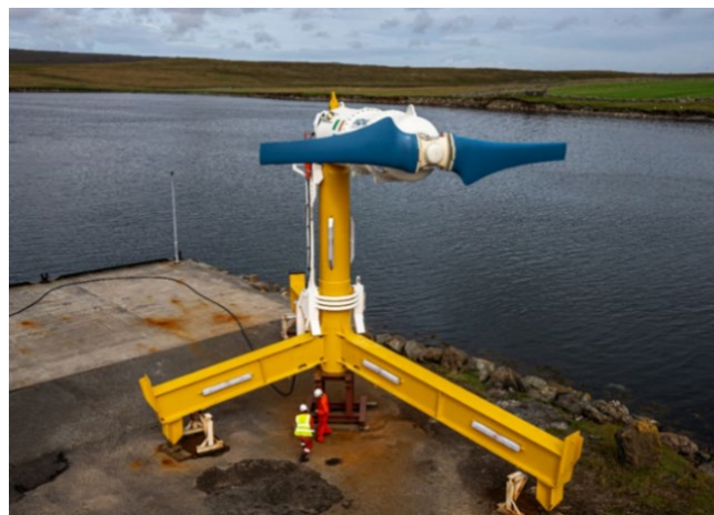
Figure 1: Nova's M100-D turbine with its substructure being prepared for deployment at the Shetland Tidal Array, Bluemull Sound.
