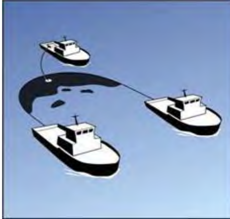
Figure C.4 - Offshore recovery boom and vessel 'U' and 'J' configurations (OSRL, 2006)
