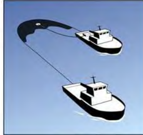
Figure C.4 - Offshore recovery boom and vessel 'U' and 'J' configurations (OSRL, 2006)
