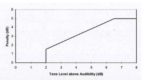
The rating level at each wind speed is the arithmetic sum of the wind farm noise level, as determined from the best fit curve described in Note 2, and the penalty for tonal noise.
