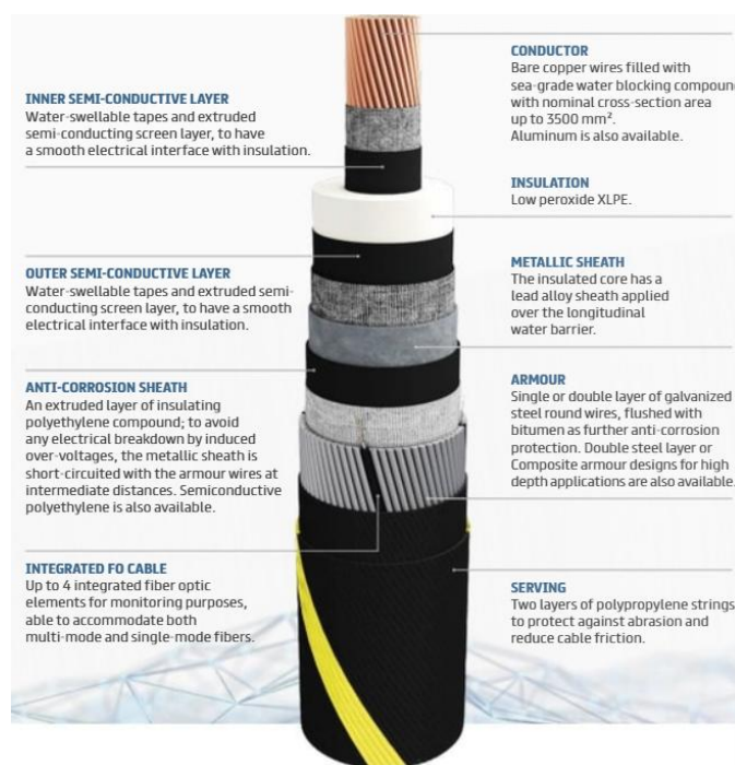
Plate 4.4 HVDC Submarine Export Cable (Prysmian, 2024)
