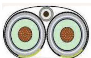
Plate 4.5 HVDC Symmetrical Monopole Bundled Cable Installation (Europacable, 2012)
