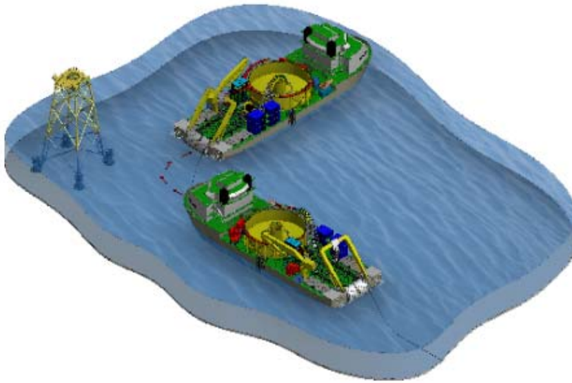
Figure 11-7: Lay vessel second end approach to structure
