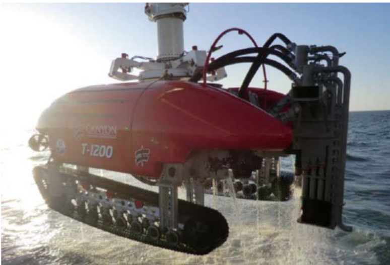
Figure 11-12: Jetting Trenching Tool (Note Jetting nozzle arms at the rear)
