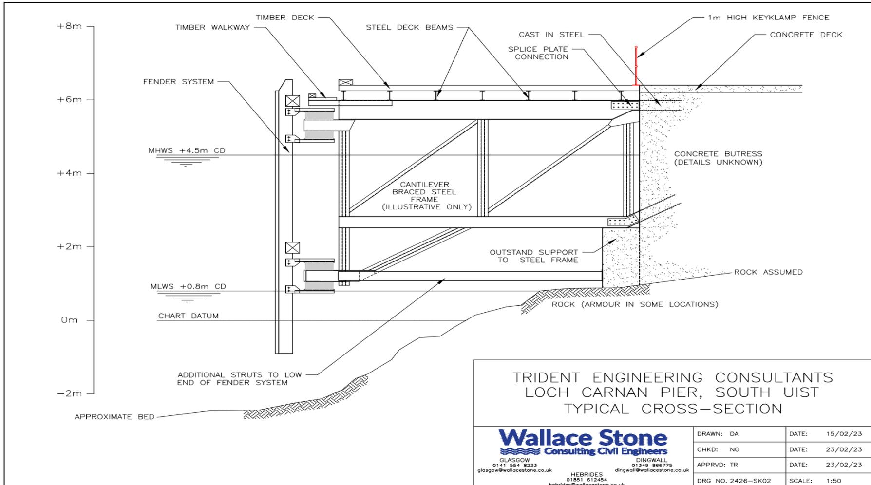
Figure 4 - Cross section of typical frame for Loch Carnan jetty
