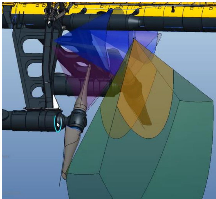
Figure 5 Potential upstream current facing camera mounting locations with indicative range shown in blue and purple cone. Final mounting locations, orientations and effective ranges will be informed through performance evaluation.
