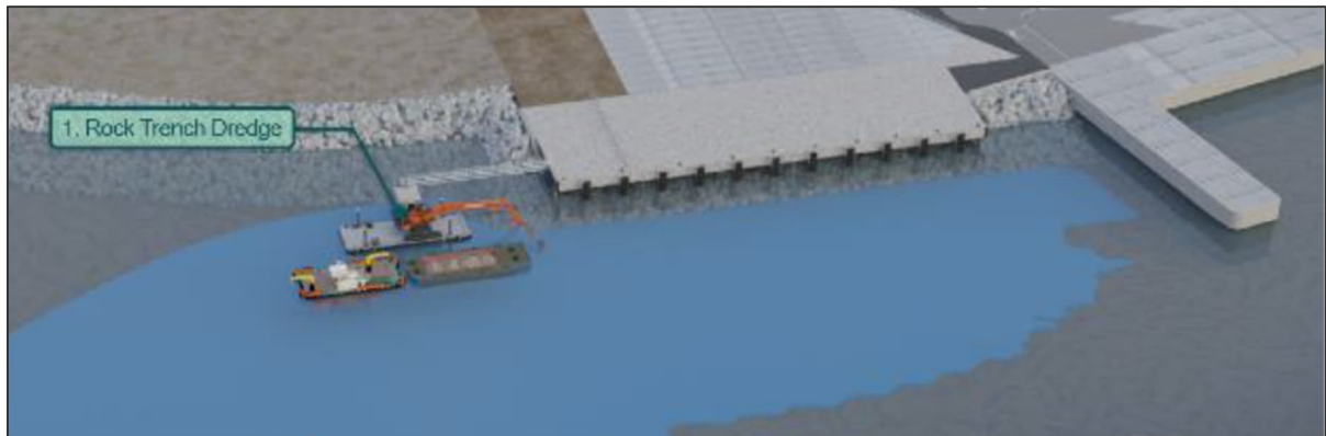
Figure 4.2 Proposed backhoe dredging of rock trench, berthing pocket, and approach.
