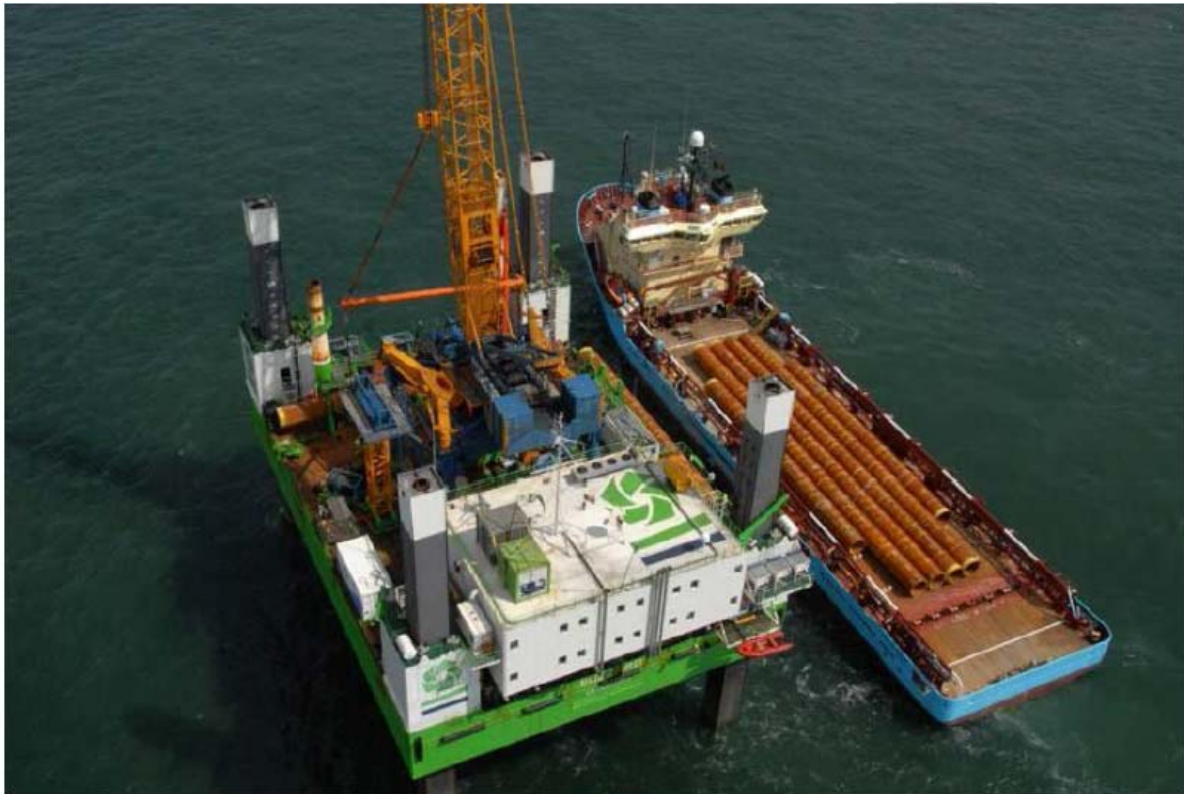
Figure 4: Example Jack Up Platform and Supply Vessel with pin piles
