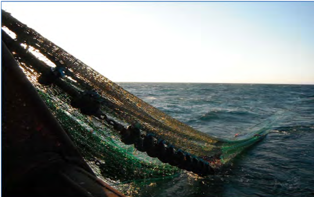
Figure 5.2 Rock-hopper otter trawl used
