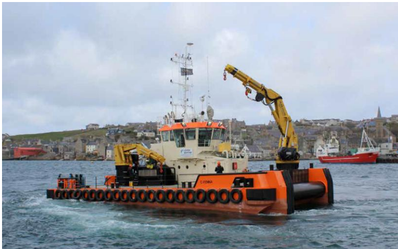
Appendix figure B-1 Example Multi Cat vessel
