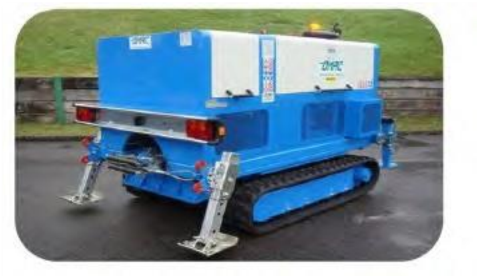
Figure 12: Tracked 10Te Bull Wheel Winch
