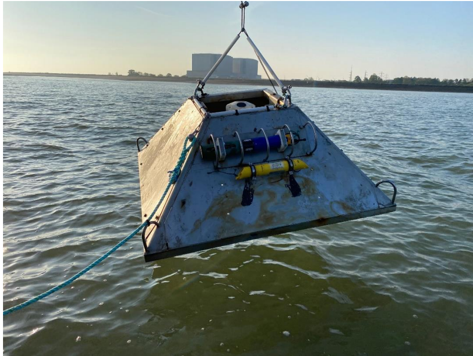
Figure 4: Example of ADCP deployed inside protection frame
