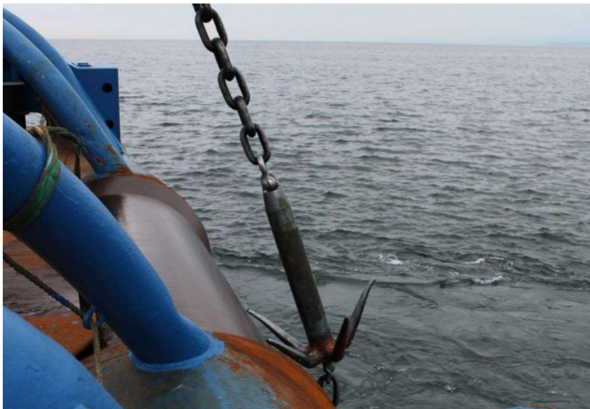
Figure 5-14 Example of grapnel and chain at stern toller of vessel
