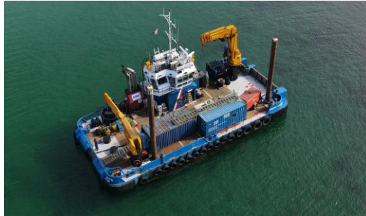
Figure 37 - Example of spud legs typically used during operations
