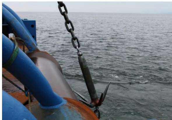
Figure 24 - Example of Grapnel and Chain at Stern Roller of Vessel
