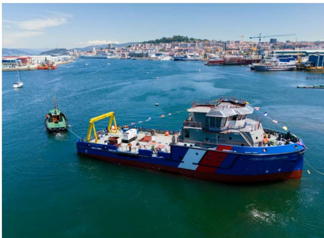
Figure 5-13 Forth Constructor - Boulder Removal, Crossing and Stabilisation Operations and Cable Lay Vessel
