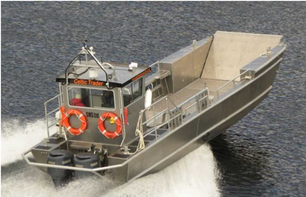
Figure 5-23 An Example Shore End Pull in Support Vessel, Celtic Trader
