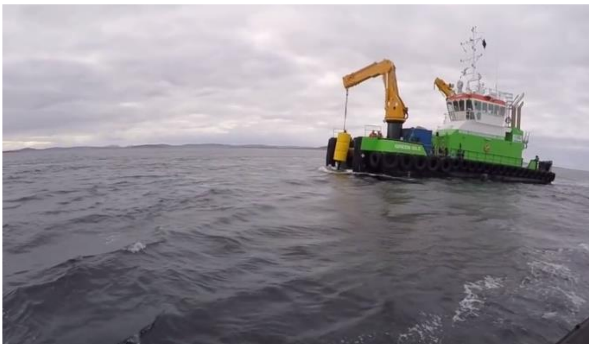
Figure 19: Installation vessel must have capacity for working with 2t buoys in tidal stream during pre-connection operations.
