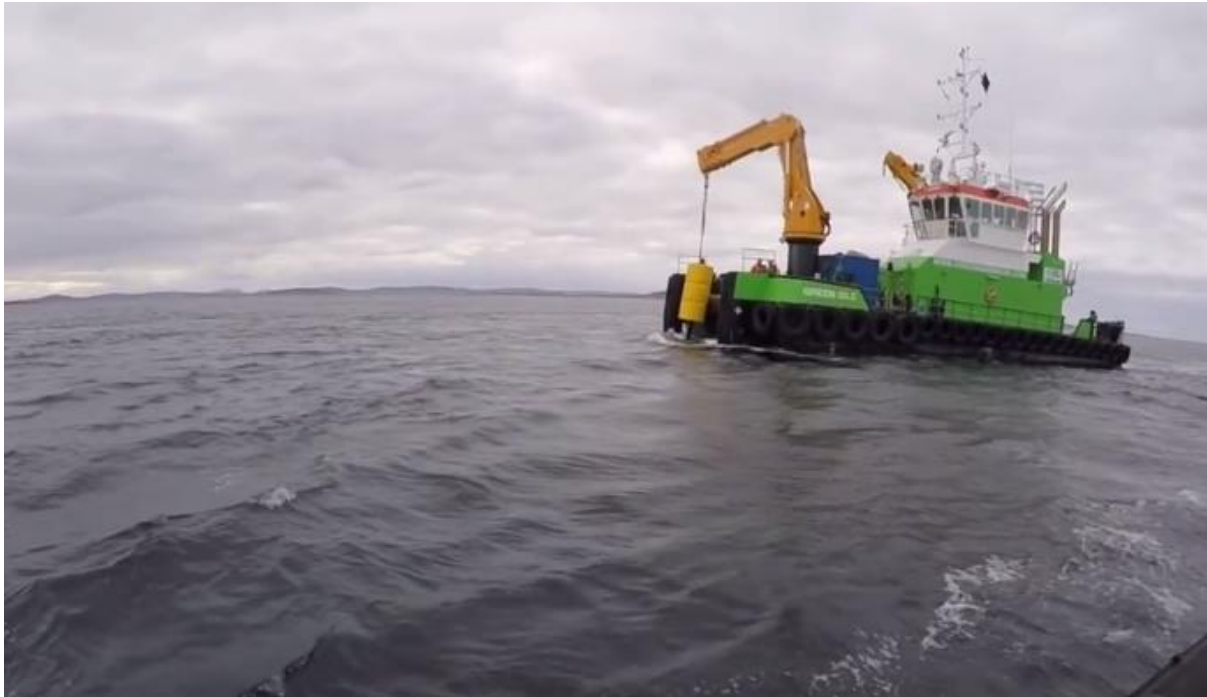
Figure 16: Installation vessel must have capacity for working with 2t buoys in tidal stream during pre-connection operations.
