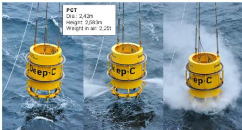
Figure 6-5: Pile cleaning tool
