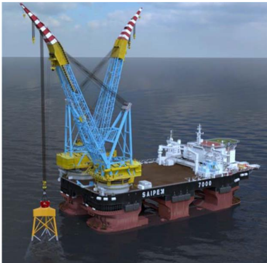
Figure 6-6: Deployment of the jacket from the SSCV
