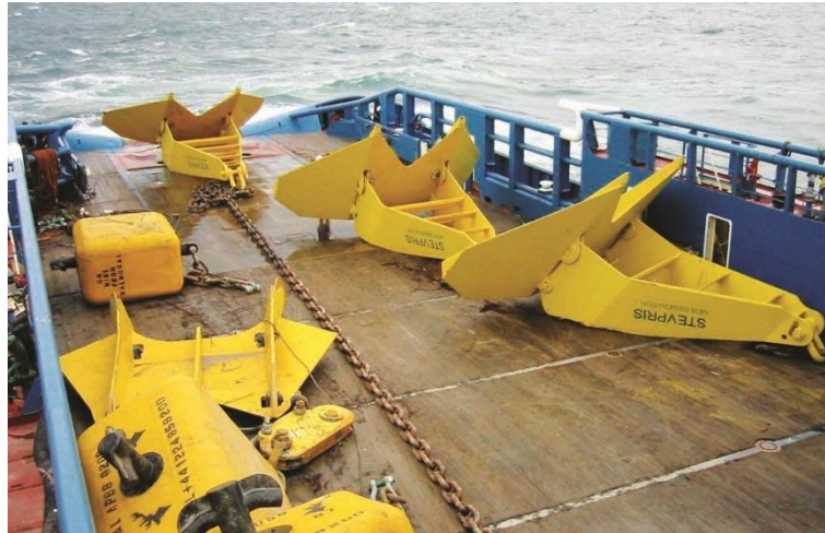
Figure 6. Drag embedment anchor
