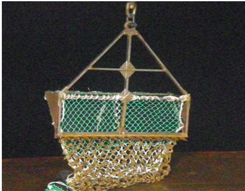
Figure 5.2 Modified 1.24m shellfish (sandeel) dredge
