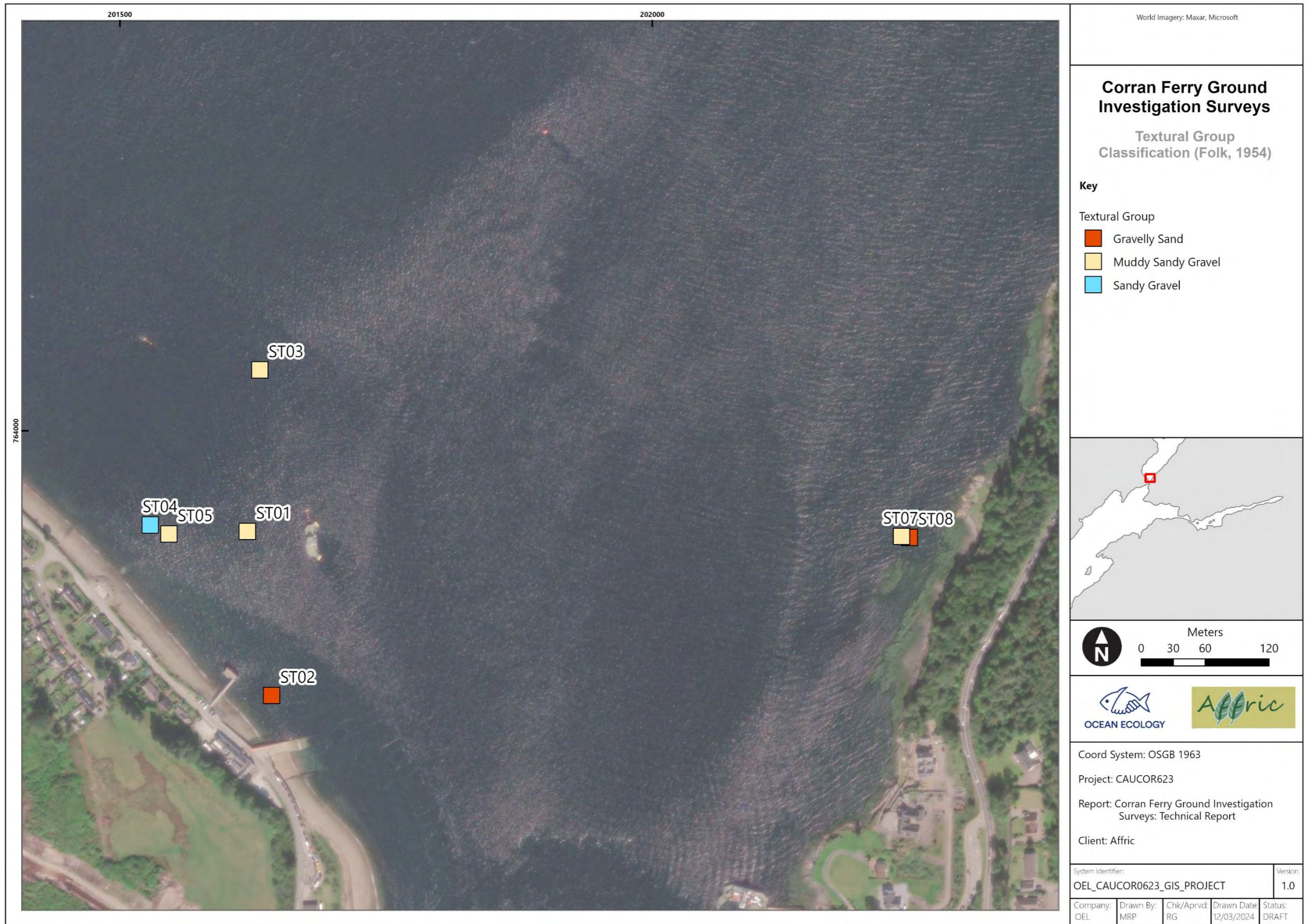
Figure 13 Textural Groups as determined from PSD analysis of samples acquired during the survey.
