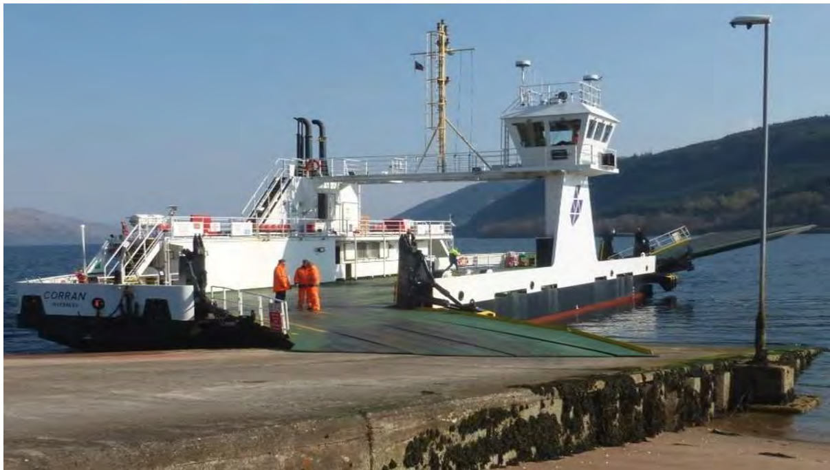
Figure 2.2.1: The MV Corran Quarter-point Vessel on the Ardgour Slipway
