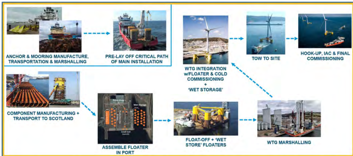
Figure 3-12: Example Foundation & WTG Construction Process Flow
