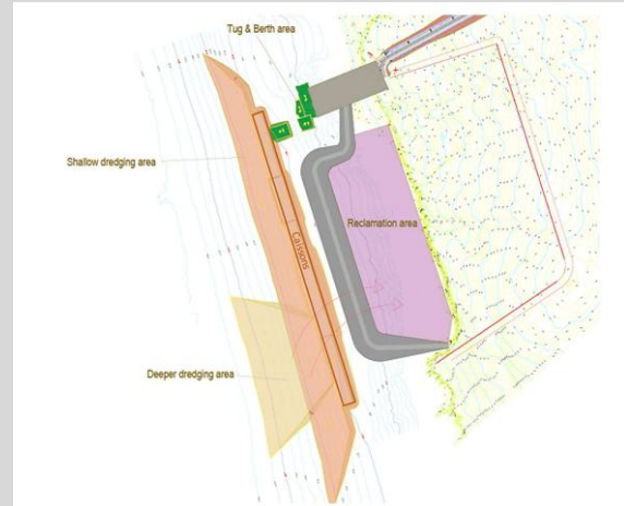
Above: Dredging and reclamation areas
