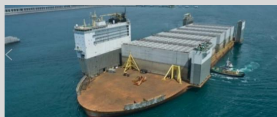
Above: Image of caisson loading operation
