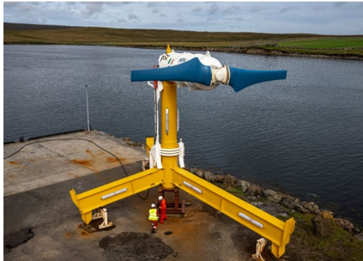
Figure 1. Nova's M100-D turbine with its substructure being prepared for deployment at the Shetland Tidal Array, Bluemull Sound. Copyright © Nova Innovation 2020
