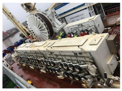
The MLV will lay away from the first shore end and bury the cable via the plough as described in Section 2.5.2.2 below. There will be certain sections (such as in areas of hard ground and at crossings (if any)) where the cable will be laid on the surface of the seabed and will not be ploughed (Section 2.5.3).
