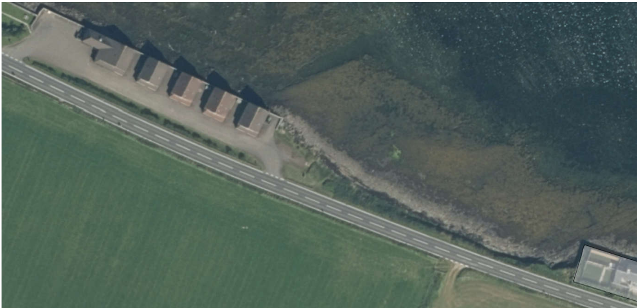
Aerial view of the site, pre development, the five Atlantis Lodges on the left, note the accretion of material to the east of the existing seawall and the shadow indicating the natural cliff line.
