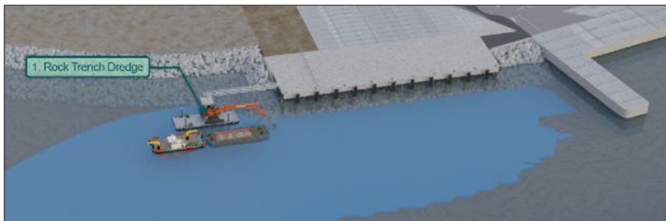
Figure 1.3 Proposed backhoe dredging of rock trench, berthing pocket, and approach.
