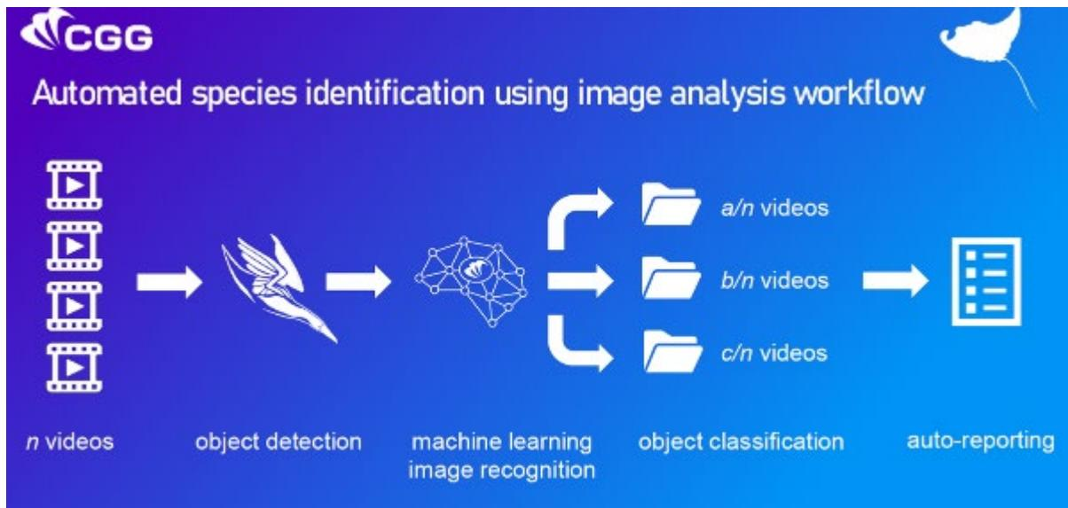
**Figure 6-1** Image analysis workflow for automated video analysis and reporting.
