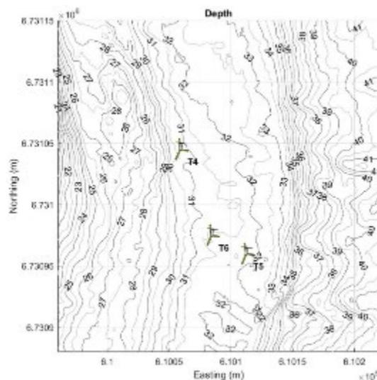
**Figure 3-2** As installed location of T4-T6 in the Shetland Tidal Array, with underlying bathymetry.
