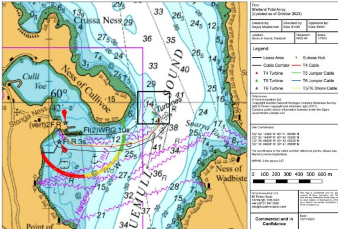
Figure 3-3 Admiralty chart showing the Shetland Tidal Array layout including turbines, hub and cables. Source: Nova Innovation 2023 © Crown Copyright
