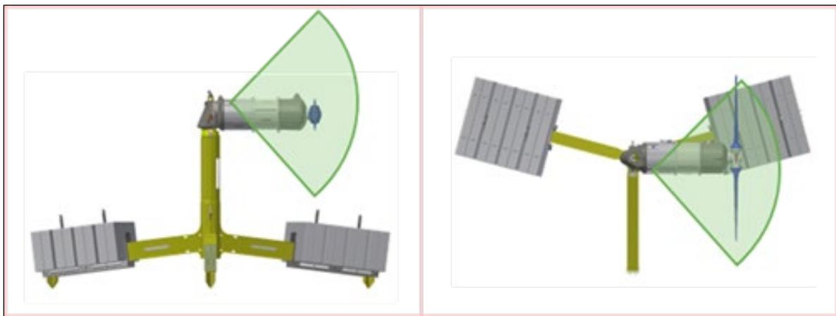
**Figure 5-1** Subsea camera system used on turbines in the Shetland Tidal Array. Camera positions and fields of views are indicative only, for illustrative purposes. Cameras are attached to the turbine nacelle.
