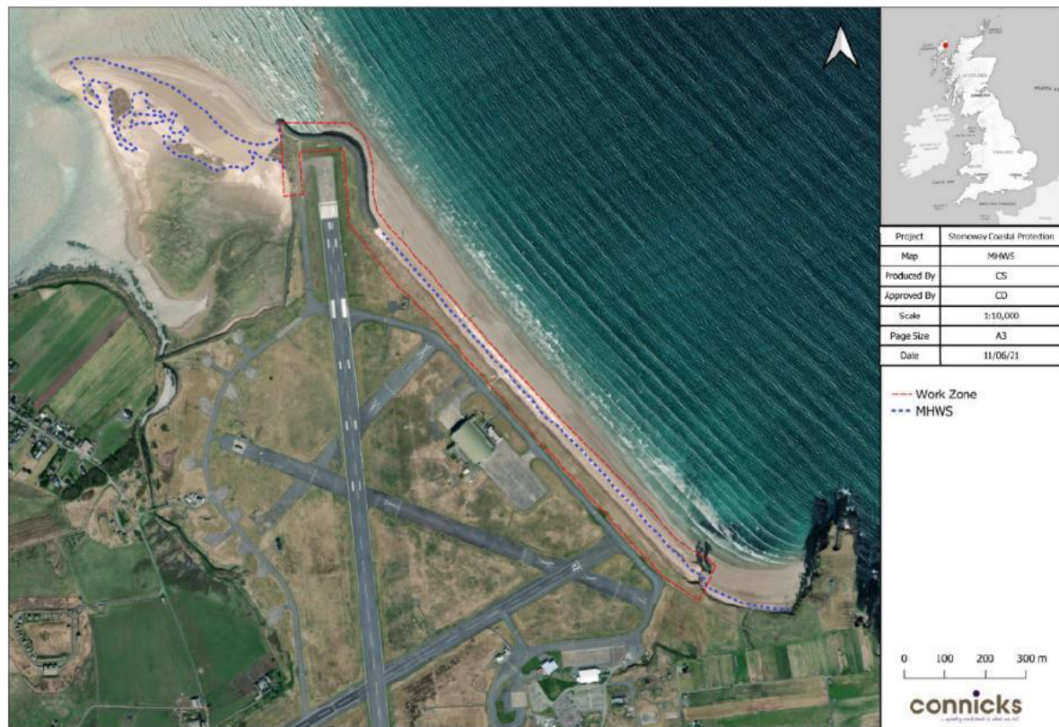
Fig 7. An aerial view of the temporary works zone overlaid with the Mean High Water Springs (Also Appendix I)
