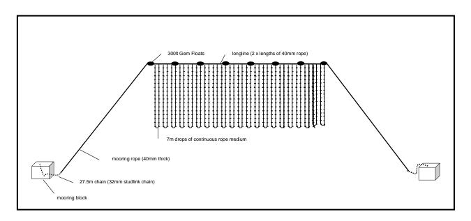
Figure 3 Longline and mooring layout – not to scale
