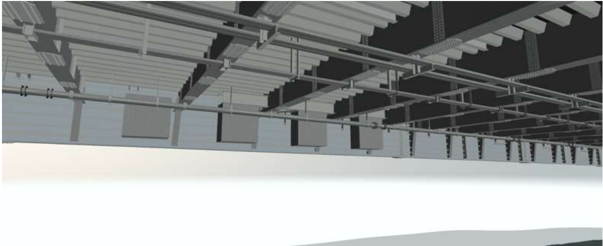
Existing TMDs under the bridge deck
