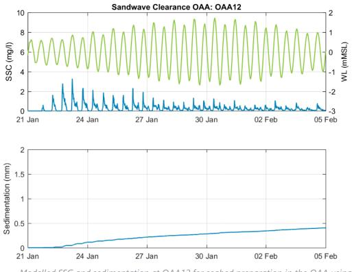
*Figure B-26* Modelled SSC and sedimentation at OAA12 for seabed preparation in the OAA using the CFE
