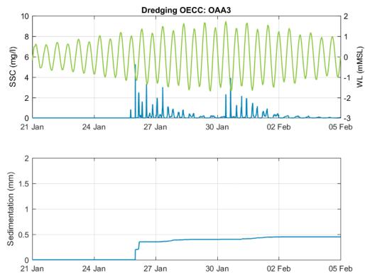
*Figure B-21* Modelled SSC and sedimentation at OAA3 as a result of placement within the indicative DMPA during for seabed preparation in the offshore ECC using a TSHD
