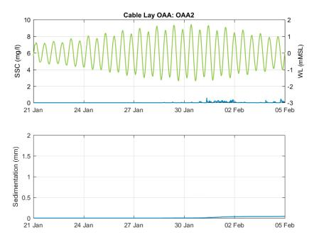
*Figure B-32* Modelled SSC and sedimentation at OAA2 for cable burial in the OAA using the CFE.
