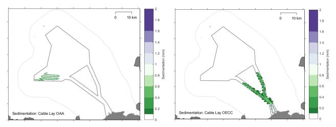
Figure 5-16 Modelled sedimentation associated with cable installation by CFE within the OAA and offshore ECC
