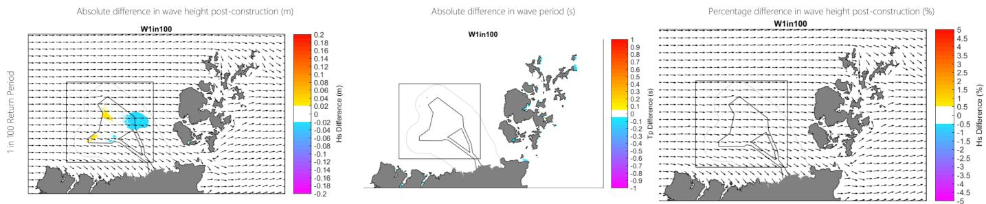
Figure B-82 Modelled change in absolute significant wave height difference (left) absolute peak period (centre) and percentage significant wave height difference (right) for layout 2 for waves approaching from the west for varying return period conditions
