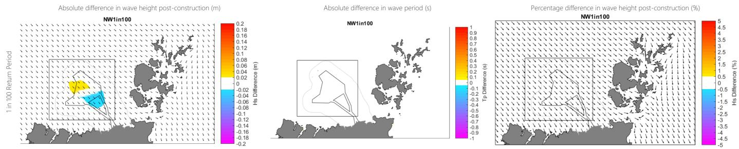
Modelled change in absolute significant wave height difference (left) absolute peak period (centre) and percentage significant wave height difference (right) for layout 1 for waves approaching from the northwest for varying return period Figure B-75 conditions
