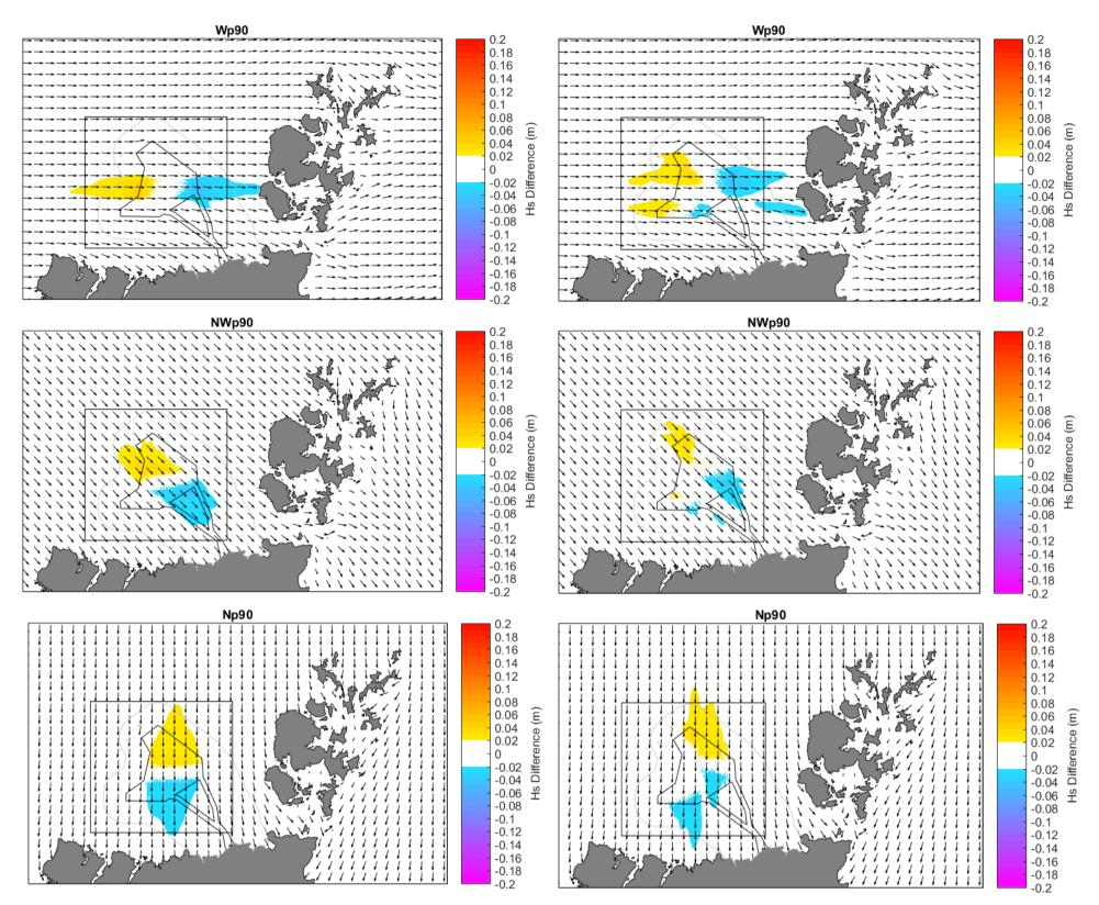
*Figure B-64* Modelled change in wave height due to layout 1 (left hand panels) and layout 2 (right hand panels) for the 90<sup>th</sup> percentile wave condition from the west (upper panels), north-west (middle panels) and north (lower panels).
