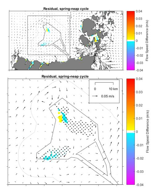
Figure 6-2 Modelled post-construction residual flows with respect to Layout 2, results are for the model domain (top) and offshore Project area zoom (bottom). Colours illustrate the post-construction flow speed difference, while the vectors illustrate the baseline residual flow speed and direction<sup>12</sup>
