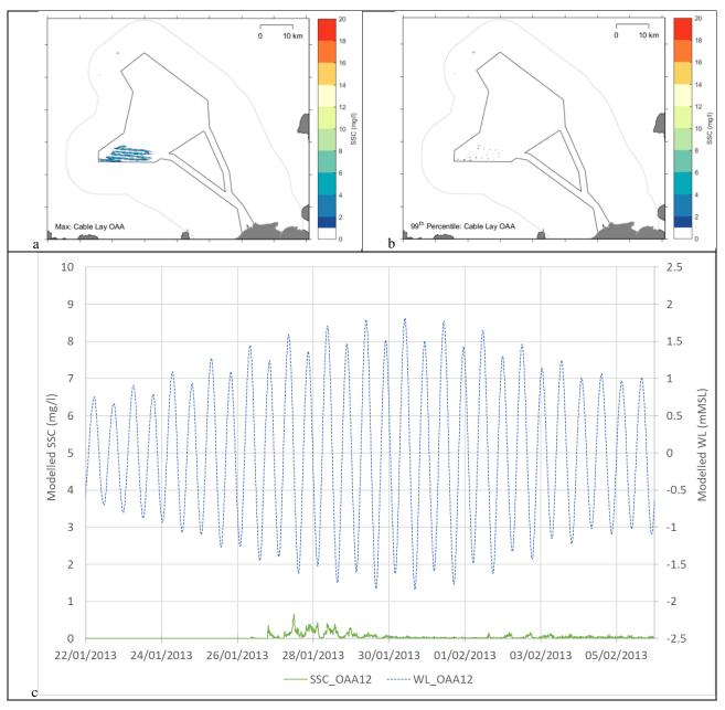
Figure 5-10 Model results for cable installation by CFE within the OAA (a) maximum plume SSC and extent modelled across the 16-day model period; (b) 99<sup>th</sup> percentile SSC and extent; (c) 95<sup>th</sup> percentile SSC and extent; and (d) SSC timeseries from model observation location OAA12, as illustrated in Figure 2-4
