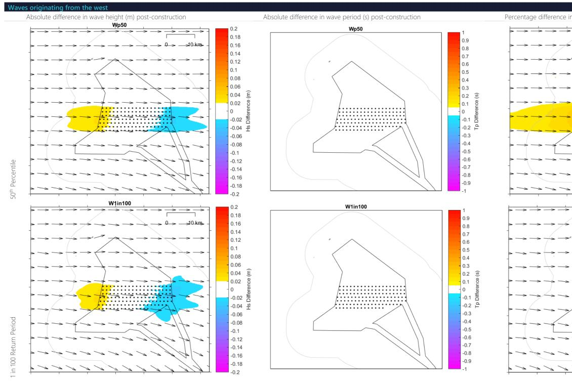
*Figure 6-5 Potential change in waves originating from the west post-construction (Layout 1)*
