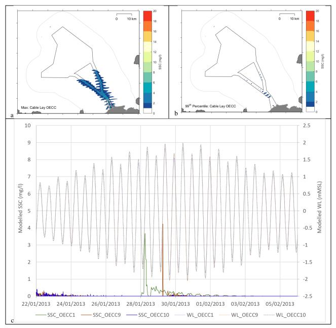
Figure 5-11 Model results for cable installation by CFE within the offshore ECC (a) maximum plume SSC and extent modelled across the 16-day model period; (b) 99<sup>th</sup> percentile SSC and extent; (c) 95<sup>th</sup> percentile SSC and extent; and (d) SSC timeseries from model observation location ECC1, ECC9 and ECC10, as illustrated in Figure 2-4
