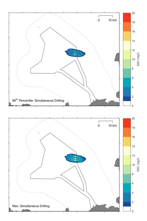
*Figure B-35* Modelled 99th percentile (top) and maximum (bottom) SSC from the PT model simulation for monopile drilling at two structures at a time.
