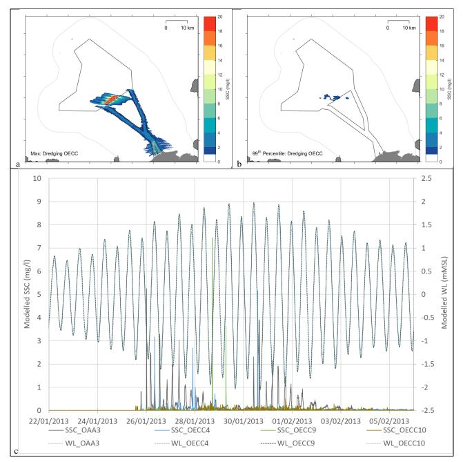
Figure 5-3 Model results for dredge and disposal, with dredging of the offshore ECC and disposal within the DMPA, (a) maximum plume SSC and extent modelled across the 16-day model period; (b) 99<sup>th</sup> percentile SSC and extent and (c) SSC timeseries from model observation locations ECC4, ECC9, ECC10 and OAA3, as illustrated in Figure 2-4
