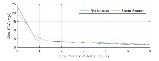
*Figure B-49 Decay in SSC plume concentration associated with pile drilling*
