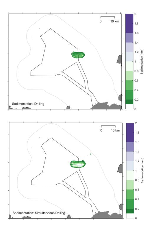
*Figure B-36* Modelled sedimentation from the PT model simulation for monopile drilling at one structure at a time (top) and two structures at once (bottom).
