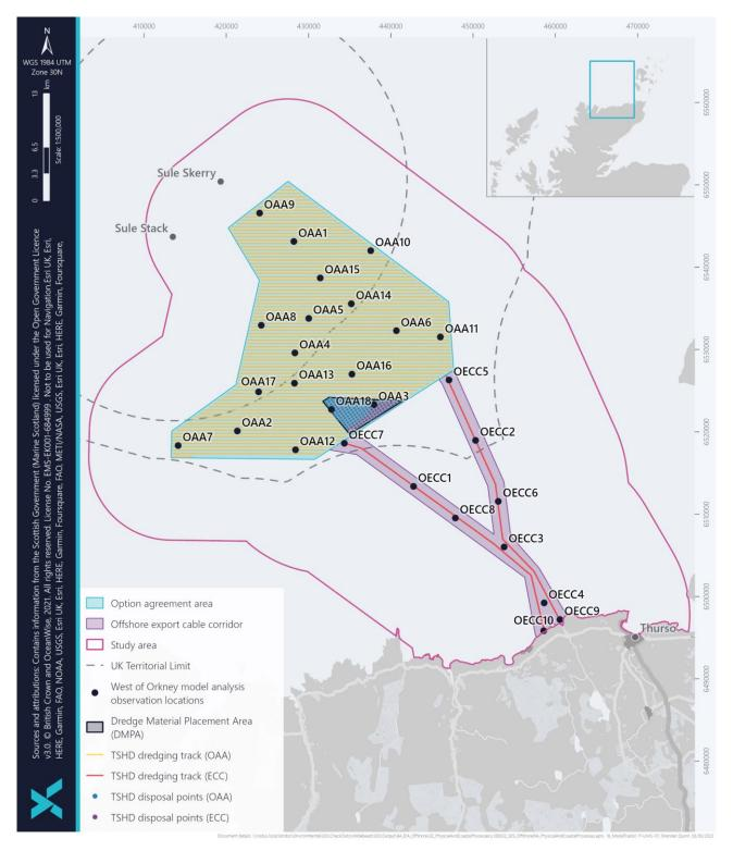
Figure 5-1 Modelled TSHD clearance track and disposal locations within the DMPA, in association with the model extraction locations, as illustrated in Figure 2-4
