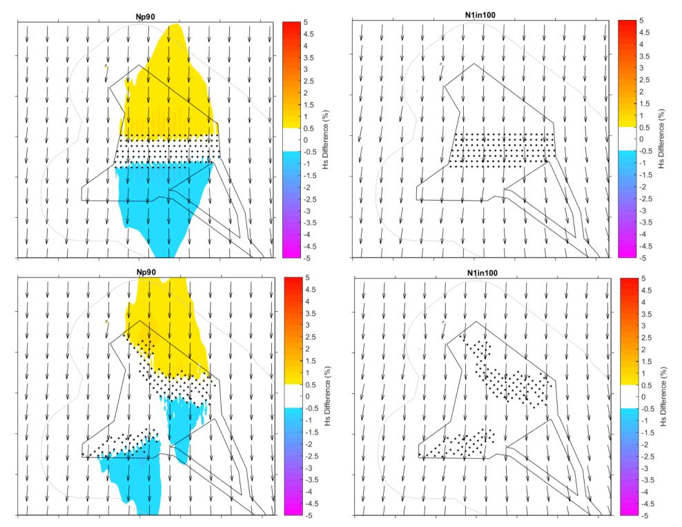
*Figure B-66* Modelled percentage change in wave height relative to the baseline conditions due to layouts 1 (top) and 2 (bottom) for the 90<sup>th</sup> percentile wave condition from the north (left hand panels) and for the 1 in 100 year ARI wave conditions from the north (right hand panels).
