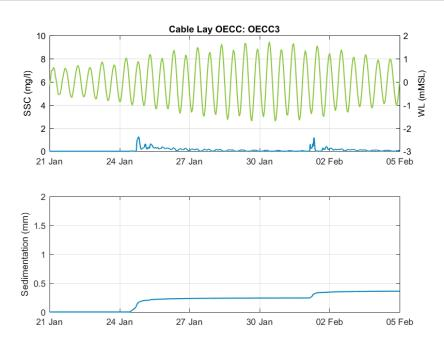
Figure B-33 Modelled SSC and sedimentation at ECC3 for cable burial in the offshore ECC using the CFE.
