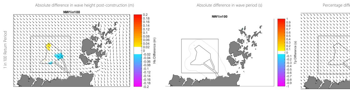
*Figure B-81* Modelled change in absolute significant wave height difference (left) absolute peak period (centre) and percentage significant wave height difference (right) for layout 2 for waves approaching from the northwest for varying return period conditions
