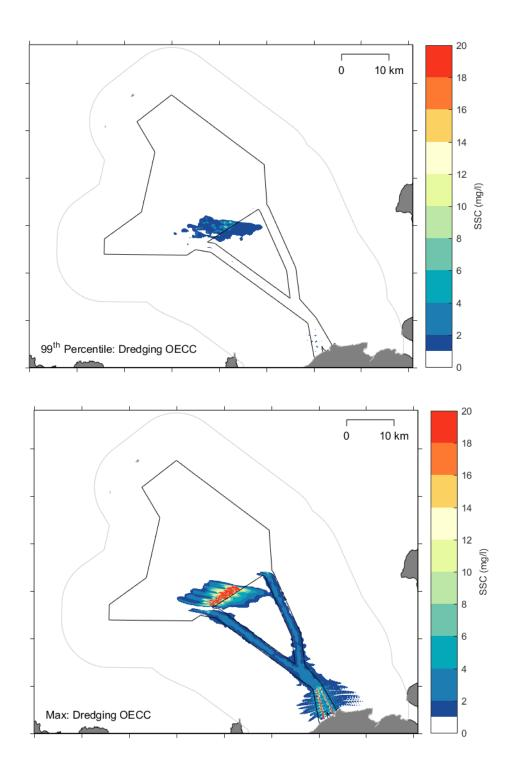
*Figure B-16* Modelled 99<sup>th</sup> percentile (top) and maximum (bottom) SSC from the PT model simulation for seabed preparation in the offshore ECC using a TSHD
