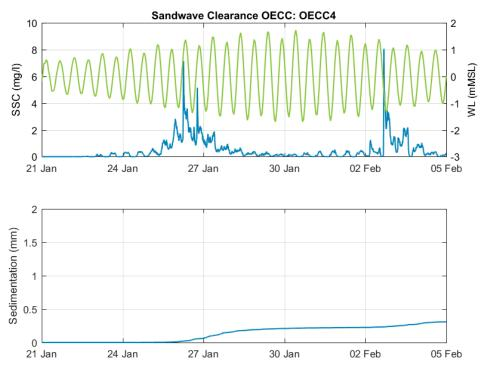
*Figure B-27* Modelled SSC and sedimentation at ECC4 for seabed preparation in the offshore ECC using the CFE
