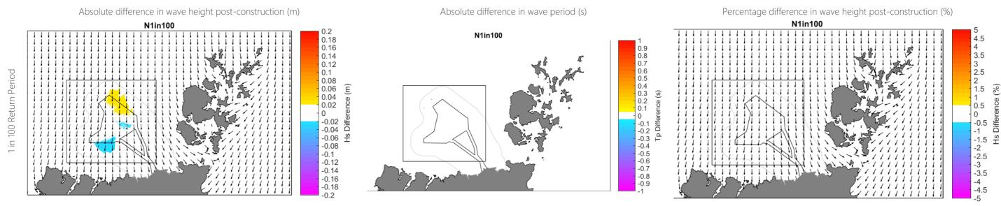
Modelled change in absolute significant wave height difference (left) absolute peak period (centre) and percentage significant wave height difference (right) for layout 2 for waves approaching from the north for varying return period Figure B-80 conditions
