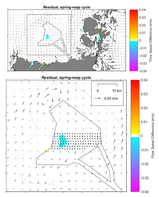
Figure 6-1 Modelled post-construction residual flows with respect to Layout 1, results are for the model domain (top) and offshore Project area zoom (bottom). Colours illustrate the post-construction flow speed difference, while the vectors illustrate the baseline residual flow speed and direction<sup>15</sup>
