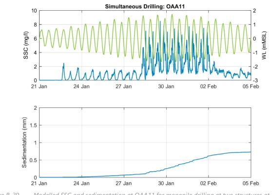
*Figure B-39 Modelled SSC and sedimentation at OAA11 for monopile drilling at two structures at a time.*
