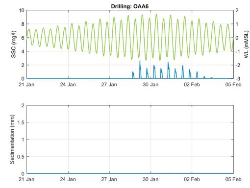
*Figure B-38* Modelled SSC and sedimentation at OAA6 for monopile drilling at one structure at a time.
