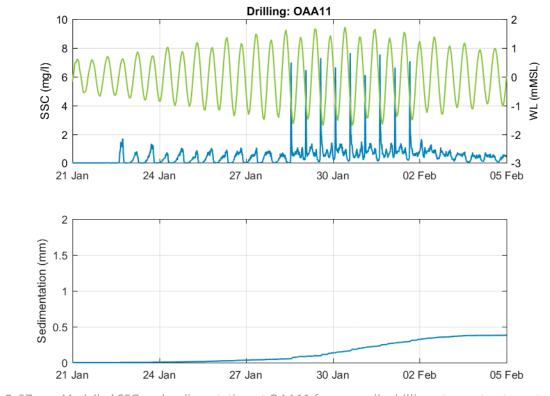
*Figure B-37 Modelled SSC and sedimentation at OAA11 for monopile drilling at one structure at a time.*
