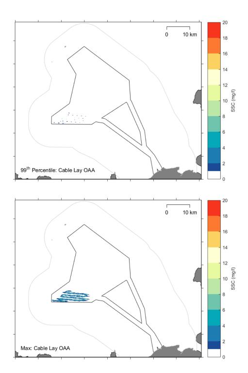
*Figure B-29* Modelled 99<sup>th</sup> percentile (top) and maximum (bottom) SSC from the PT model simulation for cable burial in the OAA using the CFE.
