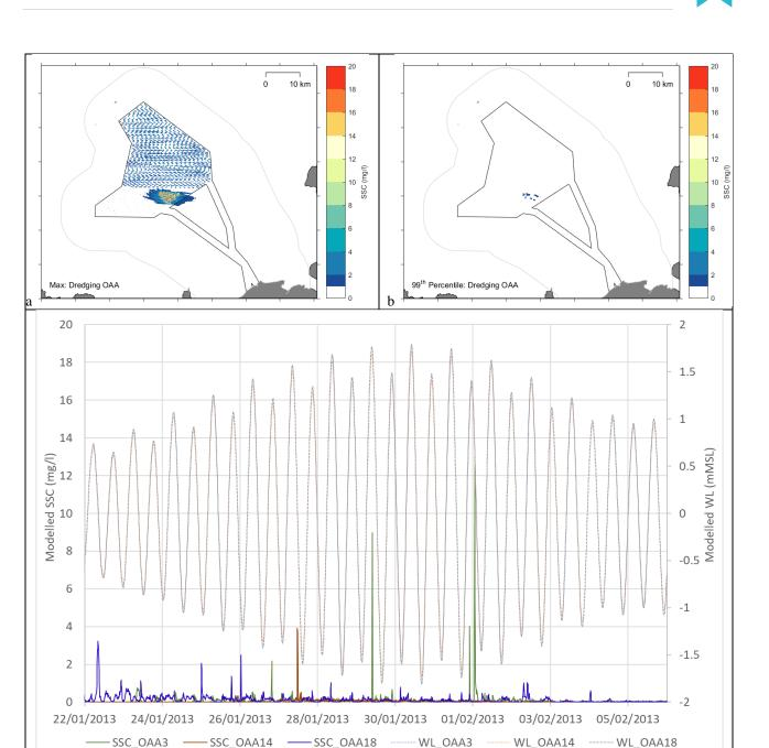
Figure 5-2 Model results for dredge and disposal for the OAA, (a) maximum plume SSC and extent modelled across the 16-day model period; (b) 99<sup>th</sup> percentile SSC and extent and (c) SSC timeseries from model observation locations OAA3, OAA14 and OAA18, as illustrated in Figure 2-4
