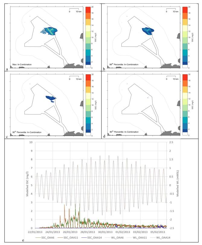
Figure 5-12 Model results for the in-combination assessment within the OAA (a) maximum plume SSC and extent modelled across the 16-day model period; (b) 99<sup>th</sup> percentile SSC and extent; (c) 95<sup>th</sup> percentile SSC and extent; (d) 80<sup>th</sup> percentile SSC and extent; and (e) SSC timeseries from model observation locations OAA6, OAA11 and OAA14, as illustrated in Figure 2-4
