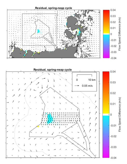
*Figure B-61* Modelled change in residual current speed over a spring neap tidal cycle for layout. Colours illustrate the post-construction flow speed difference, while the vectors illustrate the baseline residual flow speed and direction<sup>20</sup>
