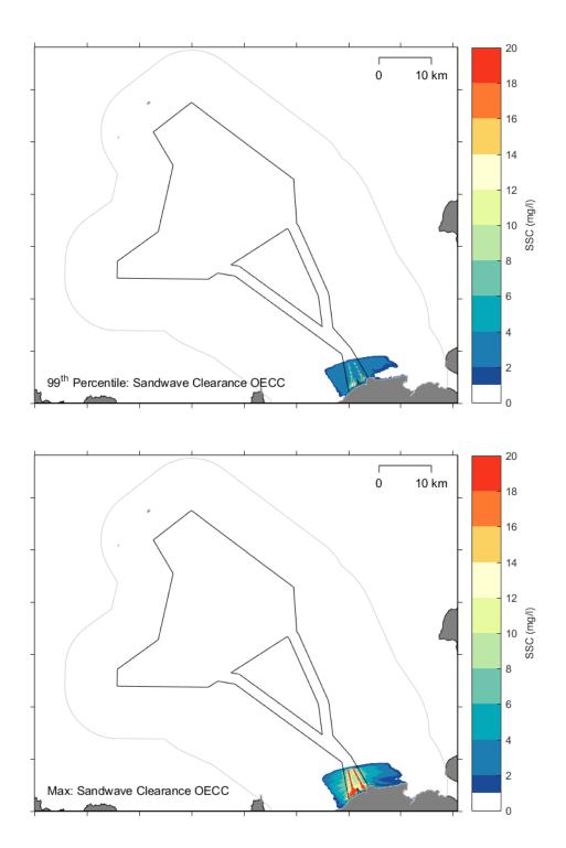
*Figure B-24* Modelled 99<sup>th</sup> percentile (top) and maximum (bottom) SSC from the PT model simulation for seabed preparation in the offshore ECC using the CFE
