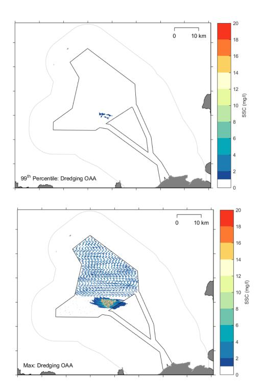
*Figure B-15* Modelled 99<sup>th</sup> percentile (top) and maximum (bottom) SSC from the PT model simulation for seabed preparation in the OAA using a TSHD
