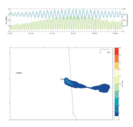
*Figure B-46 Modelled SSC from pile drilling, example plume 1 hour after drilling the second structure*
