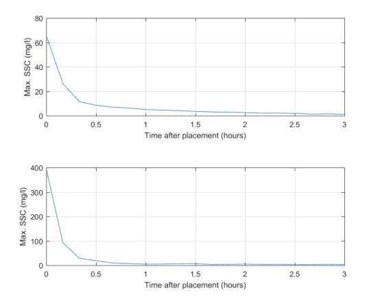
*Figure B-22* Decay in SSC placement plume concentration associated with seabed preparation in the OAA (upper) and seabed preparation in the offshore ECC (lower)
