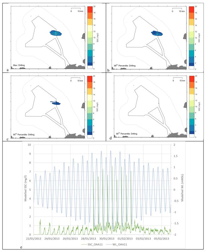
Figure 5-8 Model results for drilling of a single monopile WTG (a) maximum plume SSC and extent modelled across the 16-day model period; (b) 99<sup>th</sup> percentile SSC and extent; (c) 95<sup>th</sup> percentile SSC and extent; (d) 80<sup>th</sup> percentile SSC and extent; and (e) SSC timeseries from model observation location OAA11, as illustrated in Figure 2-4
