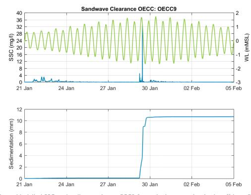
*Figure B-28* Modelled SSC and sedimentation at ECC9 for seabed preparation in the offshore ECC using the CFE
