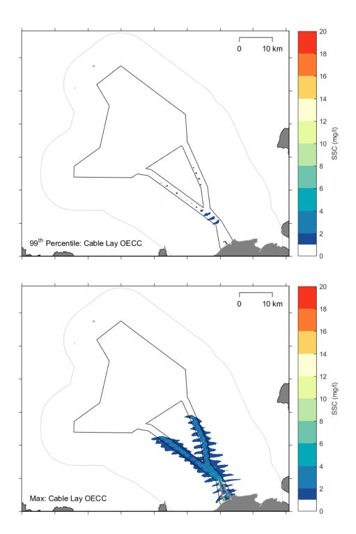
*Figure B-30* Modelled 99<sup>th</sup> percentile (top) and maximum (bottom) SSC from the PT model simulation for cable burial in the offshore ECC using the CFE.
