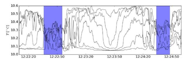
Figure 6-11 Time series of vertical temperature measurements towed past a monopile (from Shultze et al. (2020))
