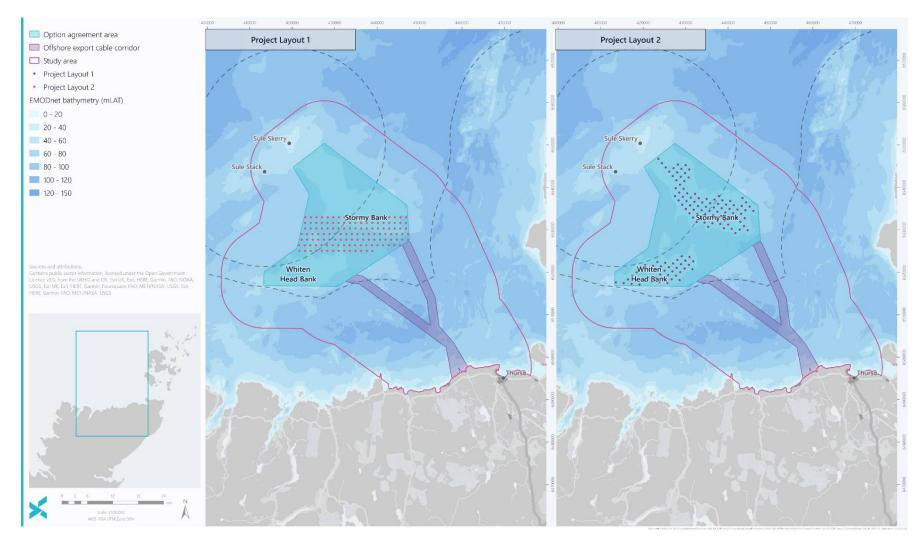
Figure 4-1 Worst case foundation layouts for marine physical and coastal processes
