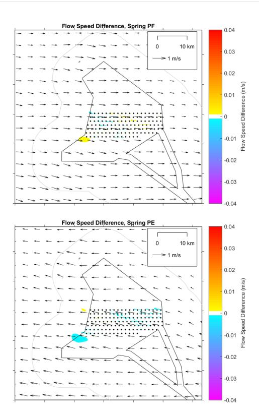
*Figure B-55* Modelled change in current speed at peak flood and peak ebb in the OAA during a mean spring tide for layout 1, zoomed across the OAA
