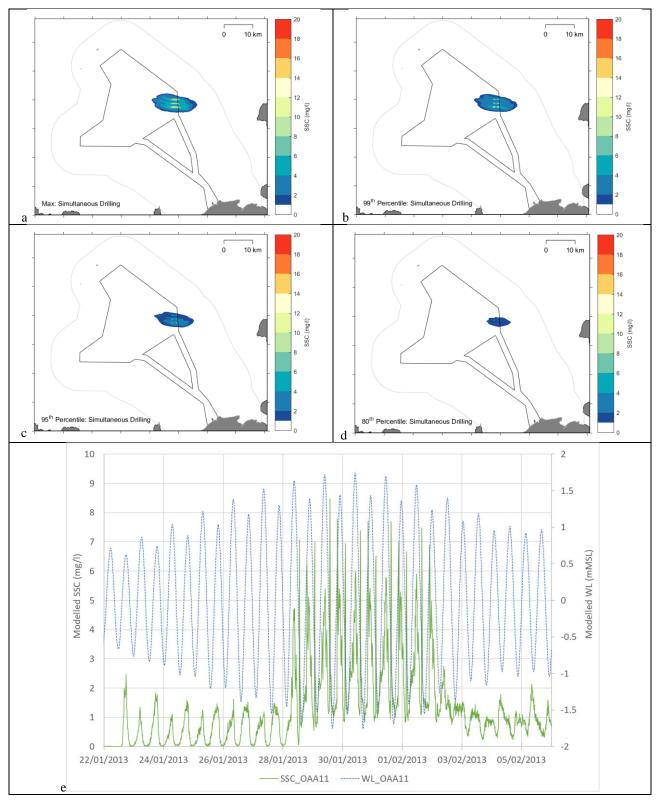
Figure 5-9 Model results for drilling two monopile WTGs concurrently (a) maximum plume SSC and extent modelled across the 16-day model period; (b) 99<sup>th</sup> percentile SSC and extent; (c) 95<sup>th</sup> percentile SSC and extent; (d) 80<sup>th</sup> percentile SSC and extent; and (e) SSC timeseries from model observation locations OAA11, as illustrated in Figure 2-4
