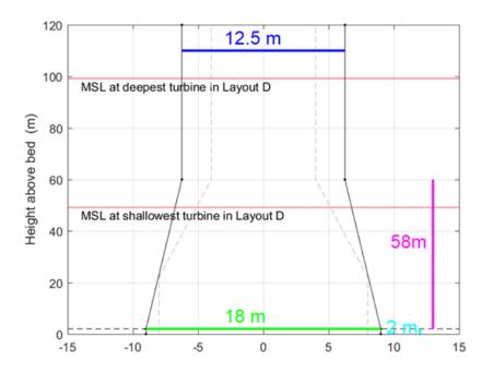
*Figure B-3* Assumed dimensions of the monopile and OSP foundations within the water column for the modelling
