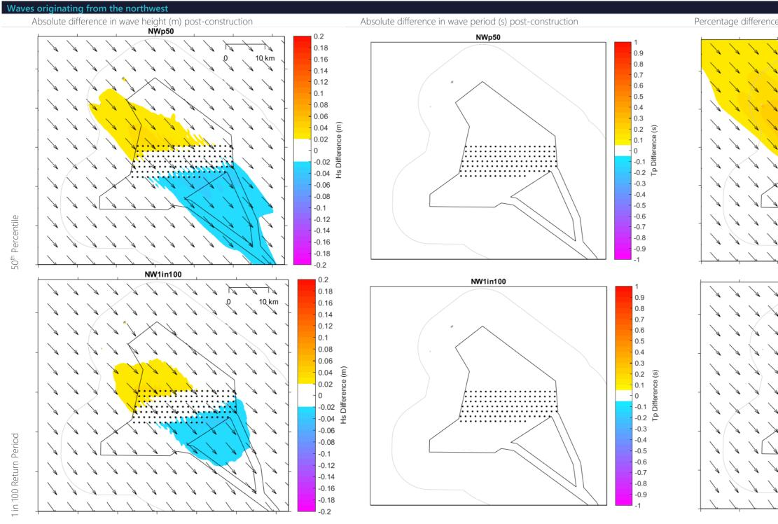
*Figure 6-4 Potential change in waves originating from the northwest post-construction (Layout 1)*
