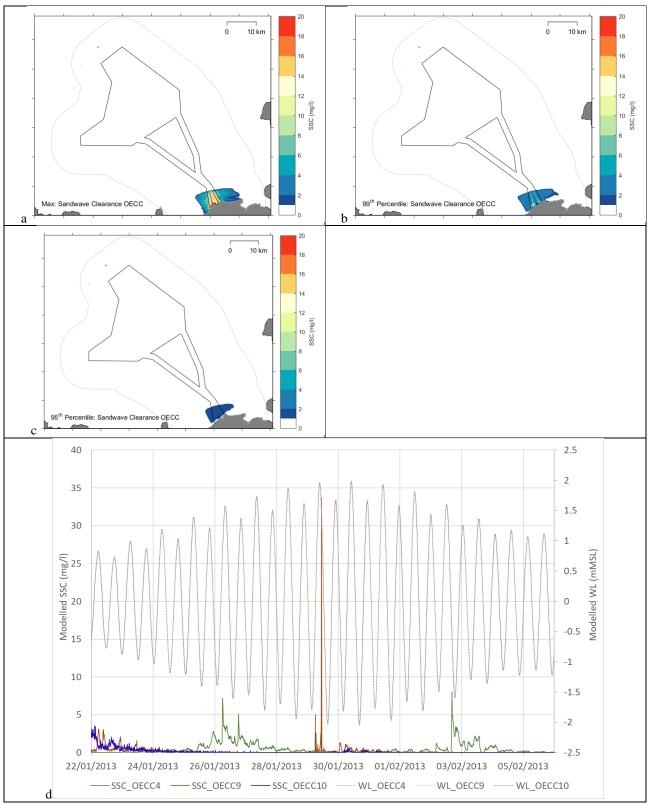
Figure 5-6 Model results for the CFE clearance within the offshore ECC, (a) maximum plume SSC and extent modelled across the 16-day model period; (b) 99<sup>th</sup> percentile SSC and extent; (c) 95<sup>th</sup> percentile SSC and extent; and (d) SSC timeseries from model observation locations ECC4, ECC9 and ECC10 as illustrated in Figure 2-4
