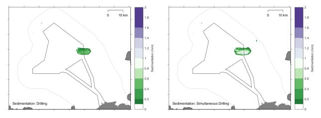
Figure 5-15 Modelled sedimentation associated with drilling one WTG monopile and two simultaneously
