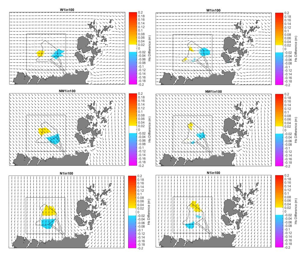
*Figure B-65* Modelled change in wave height due to layout 1 (left hand panels) and layout 2 (right hand panels) for the 1 in 100 year ARI wave condition from the west (upper panels), north-west (middle panels) and north (lower panels).
