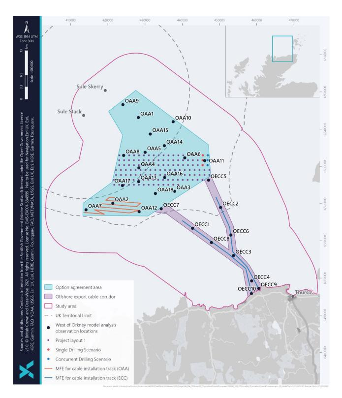
*Figure 5-7 Modelled foundation drilling (single and concurrent) and indicative cable installation tracks (inter-array/interconnectors and export), in association with the model extraction locations, as illustrated in Figure 2-4*
