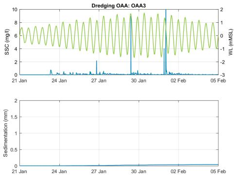
*Figure B-19* Modelled SSC and sedimentation at OAA3 as a result of placement within the indicative DMPA during seabed preparation in the OAA using a TSHD
