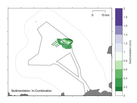
*Figure B-51* Modelled sedimentation from the in-combination construction scenario
