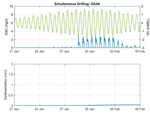
*Figure B-40* Modelled SSC and sedimentation at OAA6 for monopile drilling at two structures at a time.
