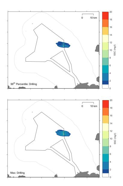
*Figure B-34* Modelled 99<sup>th</sup> percentile (top) and maximum (bottom) SSC from the PT model simulation for monopile drilling at one structure at a time.
