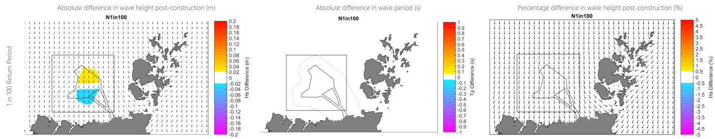
Modelled change in absolute significant wave height difference (left) absolute peak period (centre) and percentage significant wave height difference (right) for layout 1 for waves approaching from the north for varying return period Figure B-74 conditions
