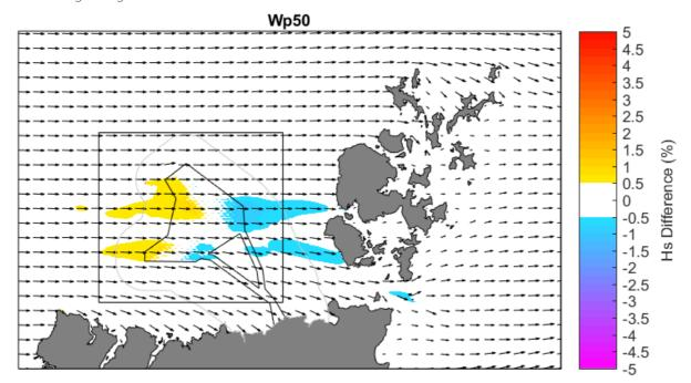
*Figure 6-10 Post-construction percentage change in significant wave height of 50<sup>th</sup> percentile waves originating from the north, northwest, and west*
