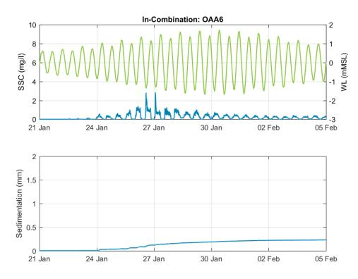
*Figure B-52* Modelled SSC and sedimentation at OAA6 the in-combination construction scenario
