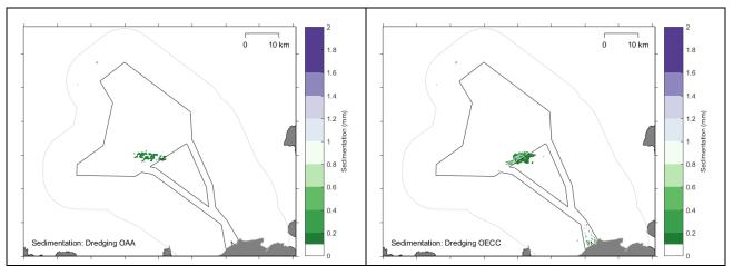
Figure 5-13 Modelled sedimentation associated with dredge and disposal clearance across the OAA and offshore ECC
