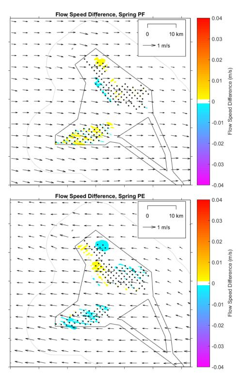
*Figure B-58* Modelled change in current speed at peak flood and peak ebb in the OAA during a mean spring tide for layout 2, zoomed across the OAA
