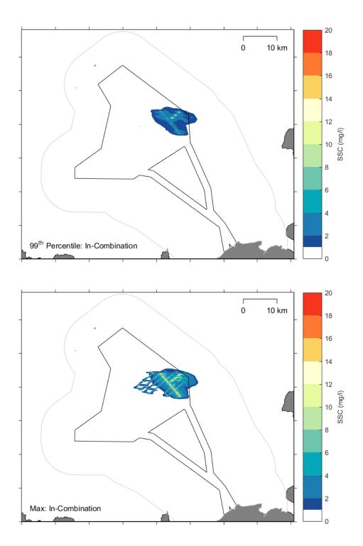
*Figure B-50* Modelled 99<sup>th</sup> percentile (top) and maximum (bottom) SSC from the in-combination construction scenario
