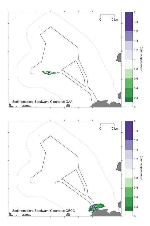
*Figure B-25* Modelled sedimentation from the PT model simulation for bedform clearance using the CFE in the OAA (top) and offshore ECC (bottom).
