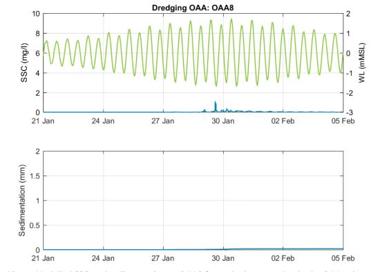
Figure B-18 Modelled SSC and sedimentation at OAA8 for seabed preparation in the OAA using a TSHD
