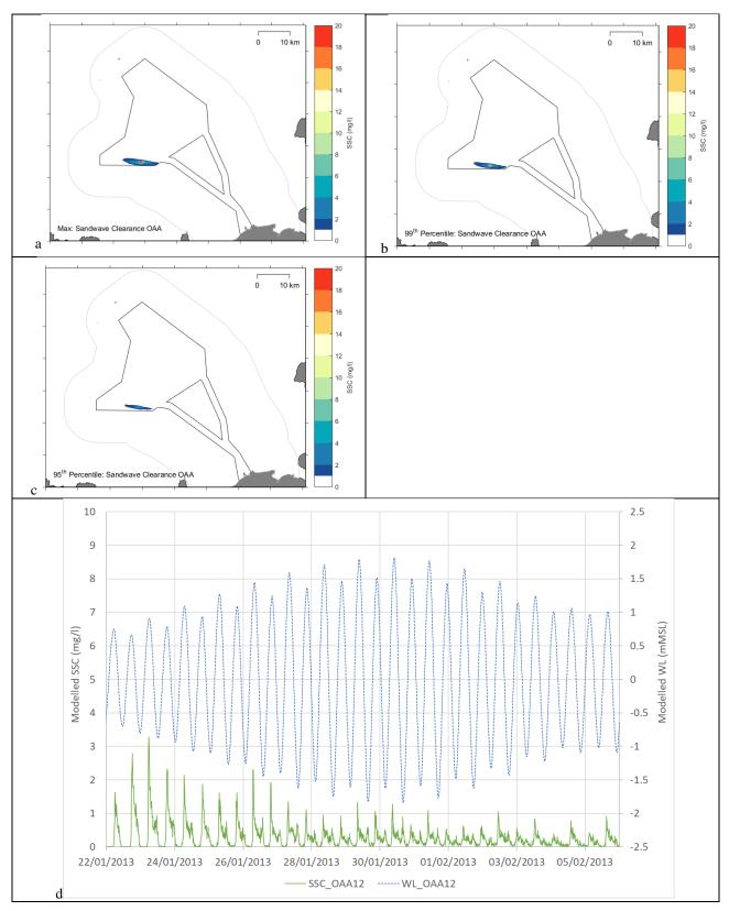
Figure 5-5 Model results for the CFE clearance within the OAA (a) maximum plume SSC and extent modelled across the 16-day model period; (b) 99<sup>th</sup> percentile SSC and extent; (c) 95<sup>th</sup> percentile SSC and extent; and (d) SSC timeseries from model observation location OAA12, as illustrated in Figure 2-4
