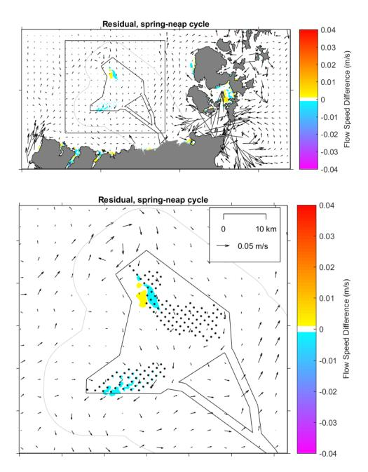
*Figure B-62* Modelled change in residual current speed over a spring neap tidal cycle for layout 2. Colours illustrate the post-construction flow speed difference, while the vectors illustrate the baseline residual flow speed and direction <sup>18</sup>
