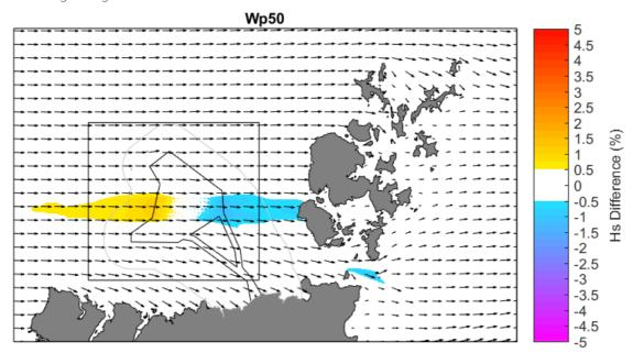
*Figure 6-6 Post-construction percentage change in significant wave height of 50<sup>th</sup> percentile waves originating from the north, northwest, and west*
