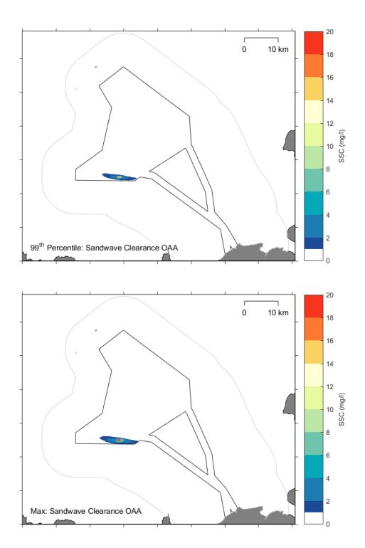
*Figure B-23* Modelled 99<sup>th</sup> percentile (top) and maximum (bottom) SSC from the PT model simulation for seabed preparation in the OAA using the CFE
