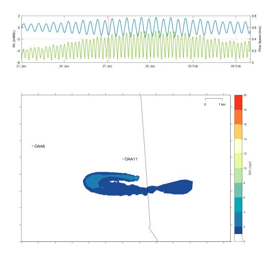
*Figure B-41* Modelled SSC from pile drilling, example plume at the end of drilling the first structure
