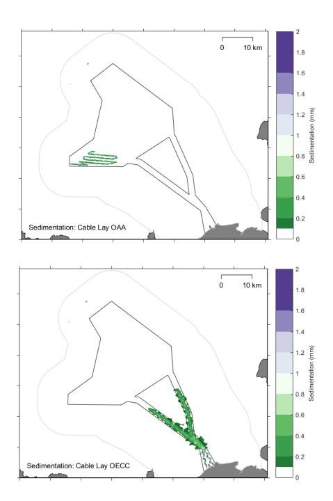
Figure B-31 Modelled sedimentation from the PT model simulation for cable burial using the CFE in the OAA (top) and offshore ECC (bottom).
