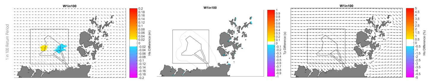
Figure B-76 Modelled change in absolute significant wave height difference (left) absolute peak period (centre) and percentage significant wave height difference (right) for layout 1 for waves approaching from the west for varying return period conditions
