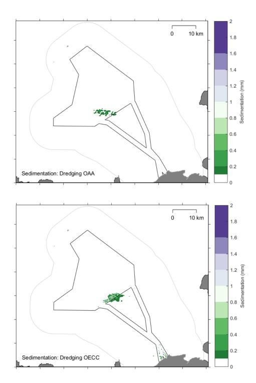
Figure B-17 Modelled sedimentation from the PT model simulation for seabed preparation in the OAA (top) and offshore ECC (bottom) using a TSHD
