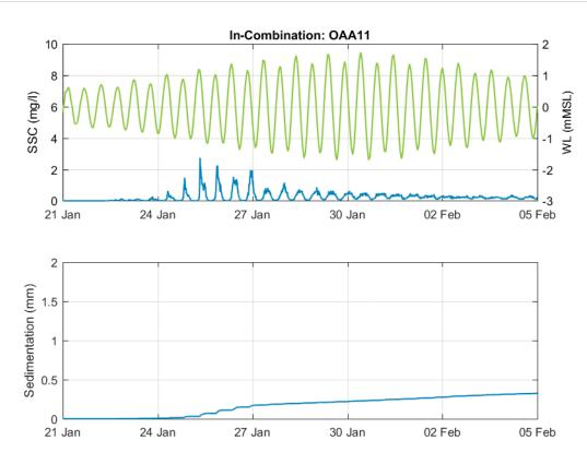
*Figure B-53* Modelled SSC and sedimentation at OAA11 the in-combination construction scenario
