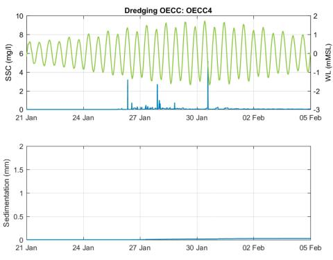
Figure B-20 Modelled SSC and sedimentation at ECC4 for seabed preparation in the offshore ECC using a TSHD
