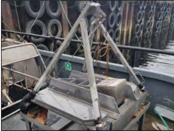
Figure 12 Hamon grab onboard the aft deck (Image Source: Survey Operational Report –, 02.22.16.OPS).
