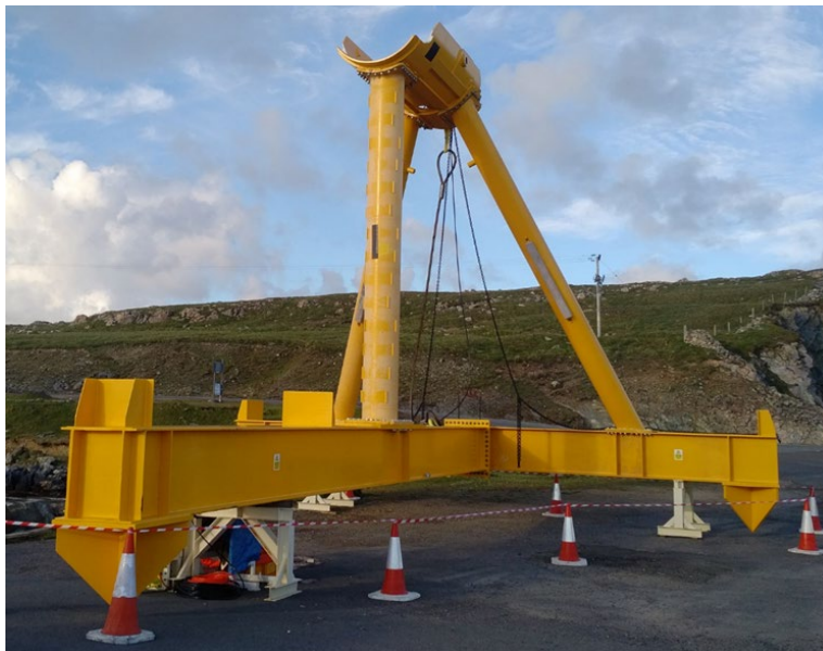
Figure 6-3: Substructure on steel trestles at Belmont pier).
