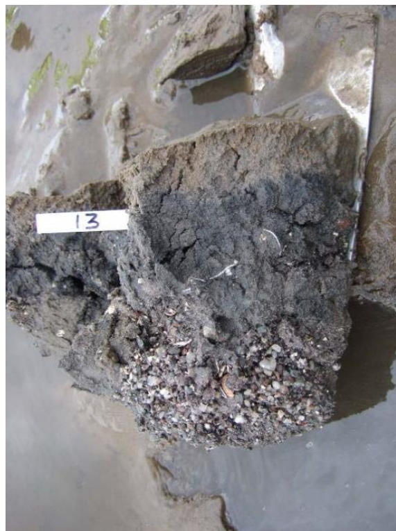
Figure 3.6: Fine Sand and Mud Deposits (0.2 m) Over Previous Beach Surface of Shelly Sand
