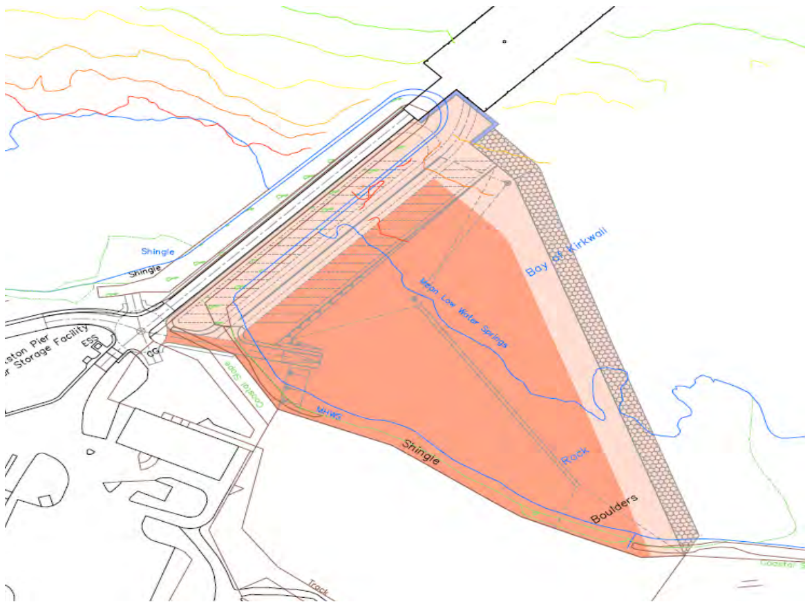
Phase 1 Reclamation – Stage 3 & 4 Complete (Area 29,600m 2 ) including sheet piled area adjacent existing suspended deck
