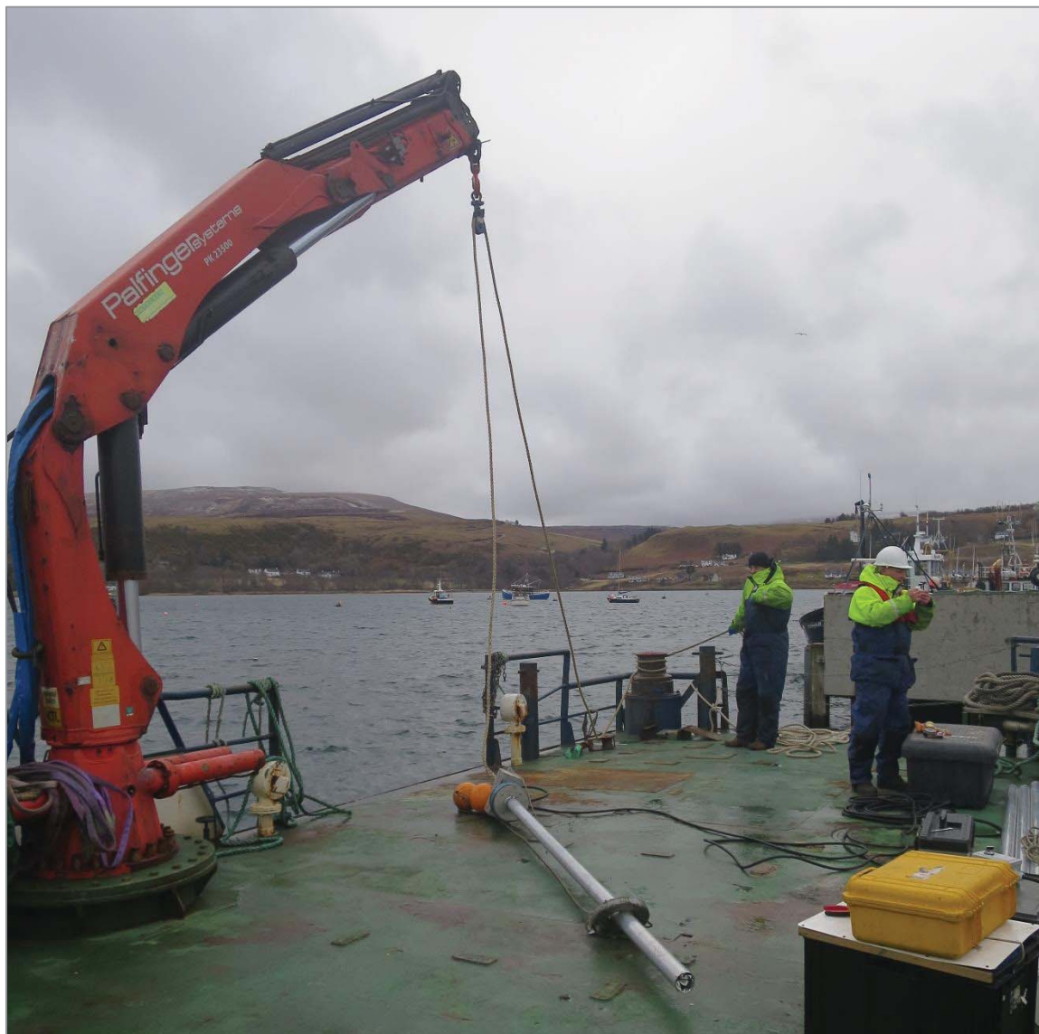
FIGURE 2 - SDI D-4 VIBROCORDER AND CORE ON DECK OF JOHANNA G
