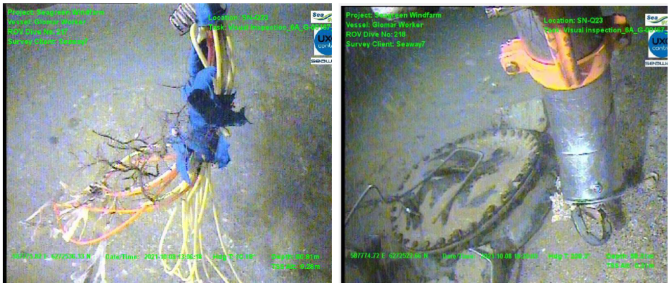
Figure 8-2: Piece of shot line and top cover plate as part of target 6A_G-00167 debris
