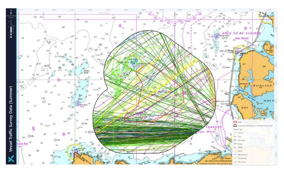
Figure 17 – Summer vessel traffic survey data within the shipping and navigation OAA study area by vessel type
