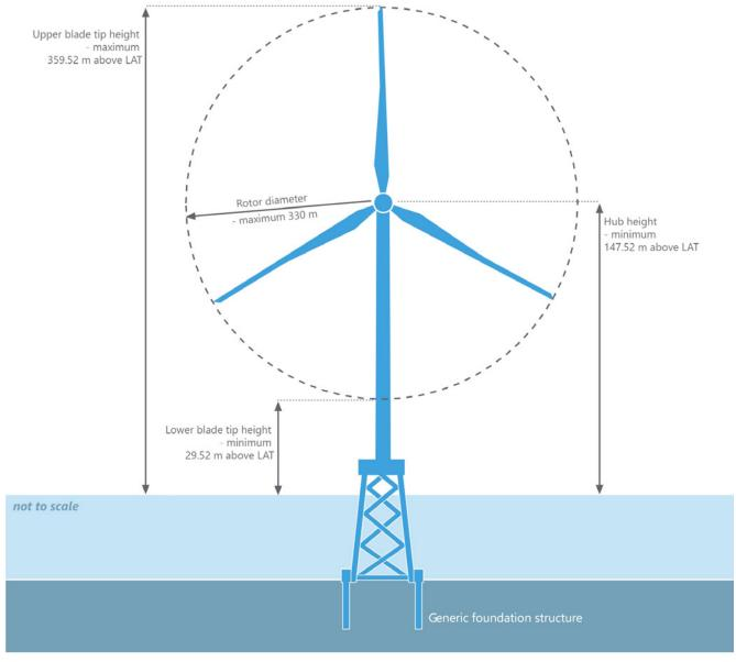
Figure 8 – Wind turbine design elements (not to scale)
