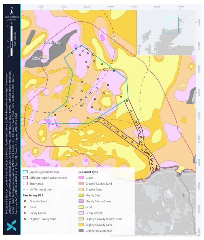
Figure 12 – Sediments across the offshore Project area comparing site specific sampling with published British Geological Society (BGS) data.
