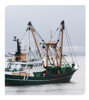
17. Larger vessels targeting crab, which have a tank with circulating seawater to keep the catch alive until it is landed.
