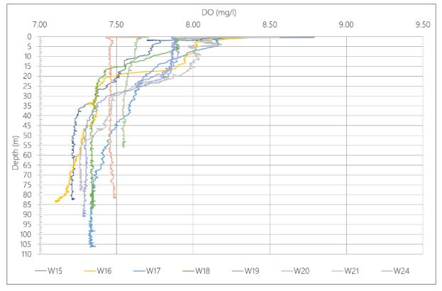
*Figure 9-8 Dissolved oxygen profiles through the water column within the OAA (top) and offshore ECC (bottom) (corresponding to locations in Figure 9-3)*
