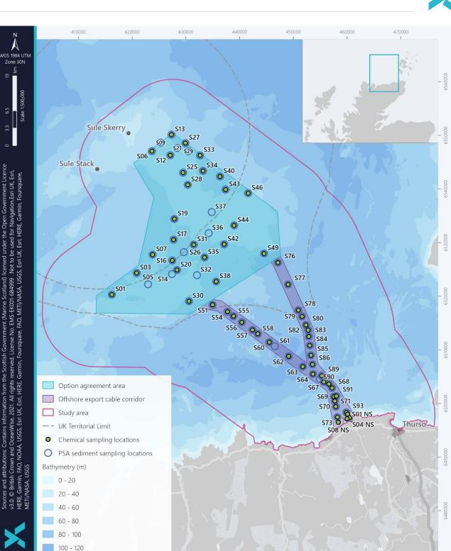
*Figure 9-2 Particle size and chemical contaminant sampled locations in the OAA and offshore ECC (see SS5: Benthic environmental baseline report)*
