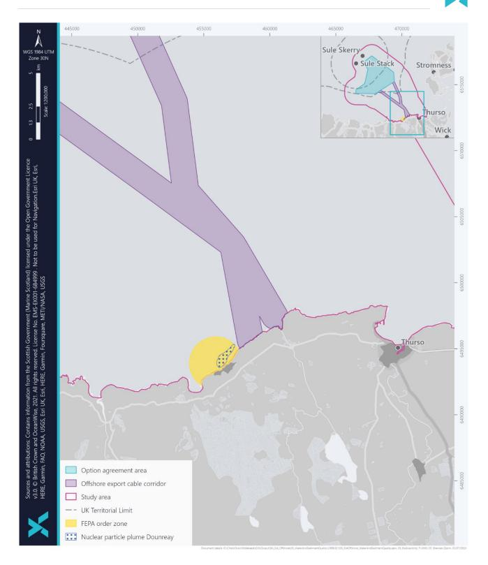
*Figure 9-15 Radioactive particles in the seabed clustered in a radioactive plume within the vicinity of the historic LEDS and the FEPA Order Zone*
