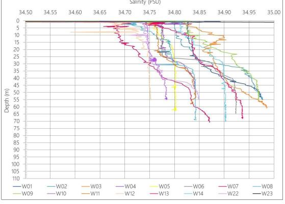
*Figure 9-4 Temperature (top) and salinity (bottom) throughout the water column within the OAA (corresponding to locations in Figure 9-3)*
