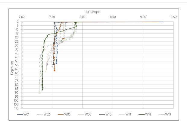
*Figure 9-10 Dissolved oxygen profiles through the water column for the replicate pairs. Colours apply to the same locations, with thicker lines for spring observations and dashed lines neap observations*
